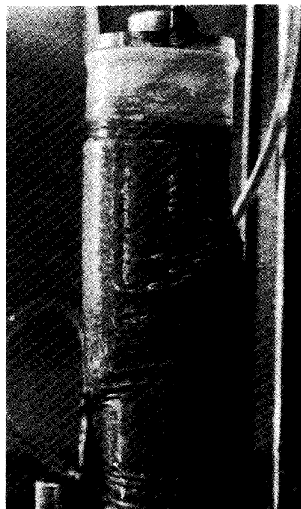
Photo 3. Typical failure mode of specimen after drained triaxial compression test, air dried condition, \sigma_3 = 3.0 \text{ kg/cm}^2
