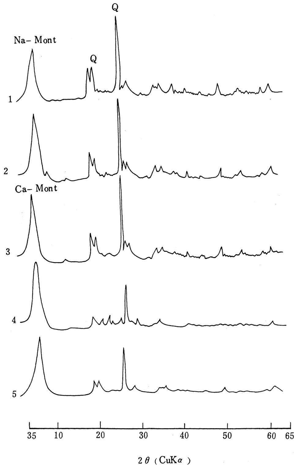
Fig. 1. X-ray powder diffraction patterns for bentonites.
