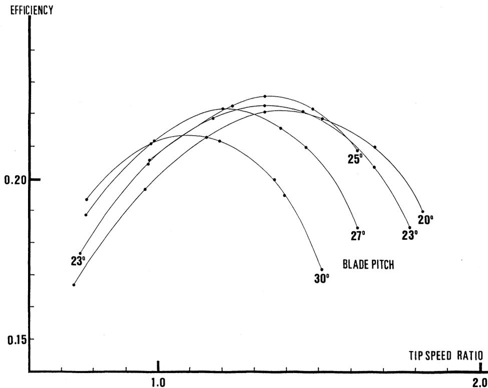
Fig. 3 Characteristic curves of efficiency. Blade pitch is angle in degree between blade plane and sweep plane. Tip speed is velocity of wing tip. Tip speed ratio is the value of tip speed by wind speed.
