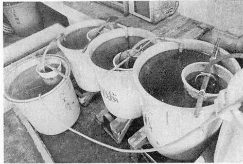
Fig. 3. Photograph showing a steady flow and calm water surfaces. (preliminary test for checking water circulation)
