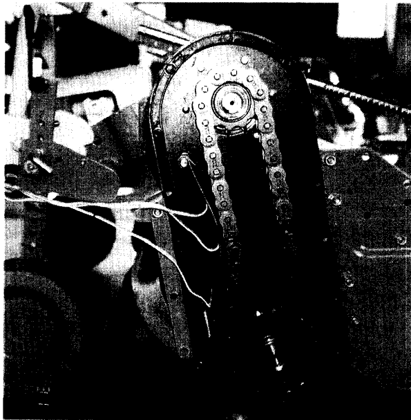
Fig. 6. Installation of the gauge attached tightener.
