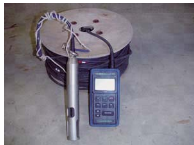
(d). Water temperature and electric conductivity meter
