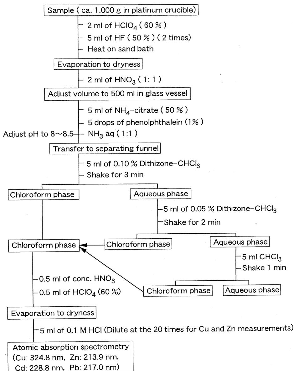
Fig. 3. Analytical procedures of copper, zinc, cadmium and lead determination for marine sediments.
