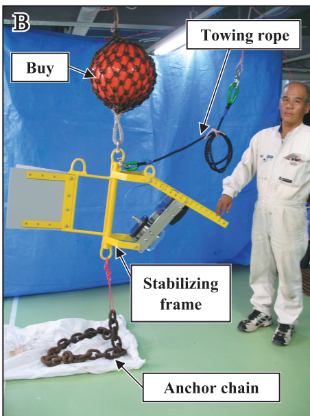
Fig. 6. Stabilizing towing device for underwater digital camera.
