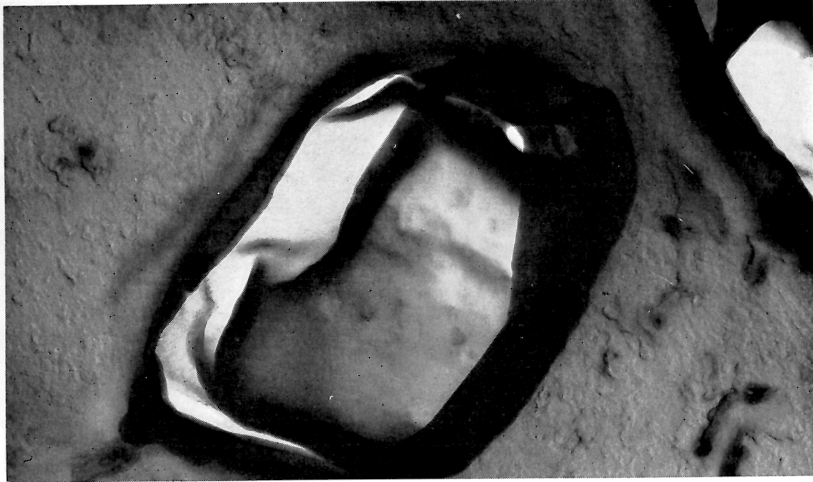
Photo. 8 1100°C×30min. w. q. after annealing at 760°C for 30min. (×20,000×2)
