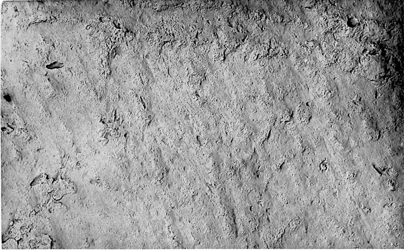
Photo. 11 350°C×30 min. w. q. after annealing at 760°C for 30 min. (×10,000×2)
