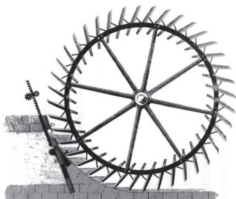
Fig.7 Modern western style chest shot water mill (17)
