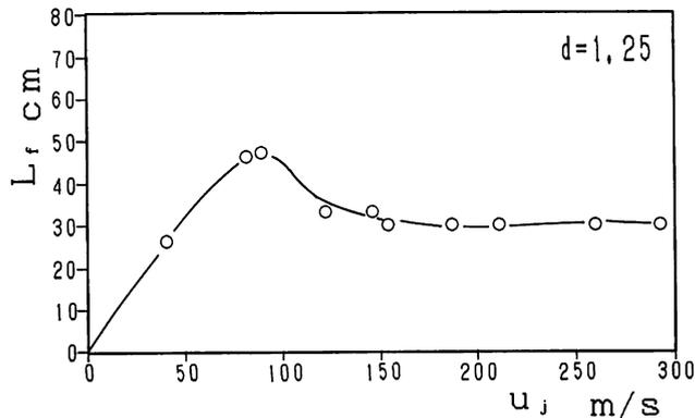
Fig. 3 Nozzle velocity versus flame length for  $d = 1.25$  mm
