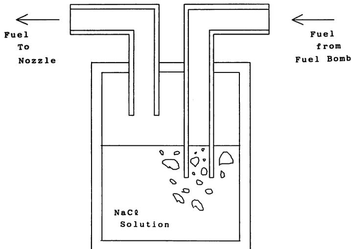
Fig. 2 A schematic of the NaCl solution vessel
