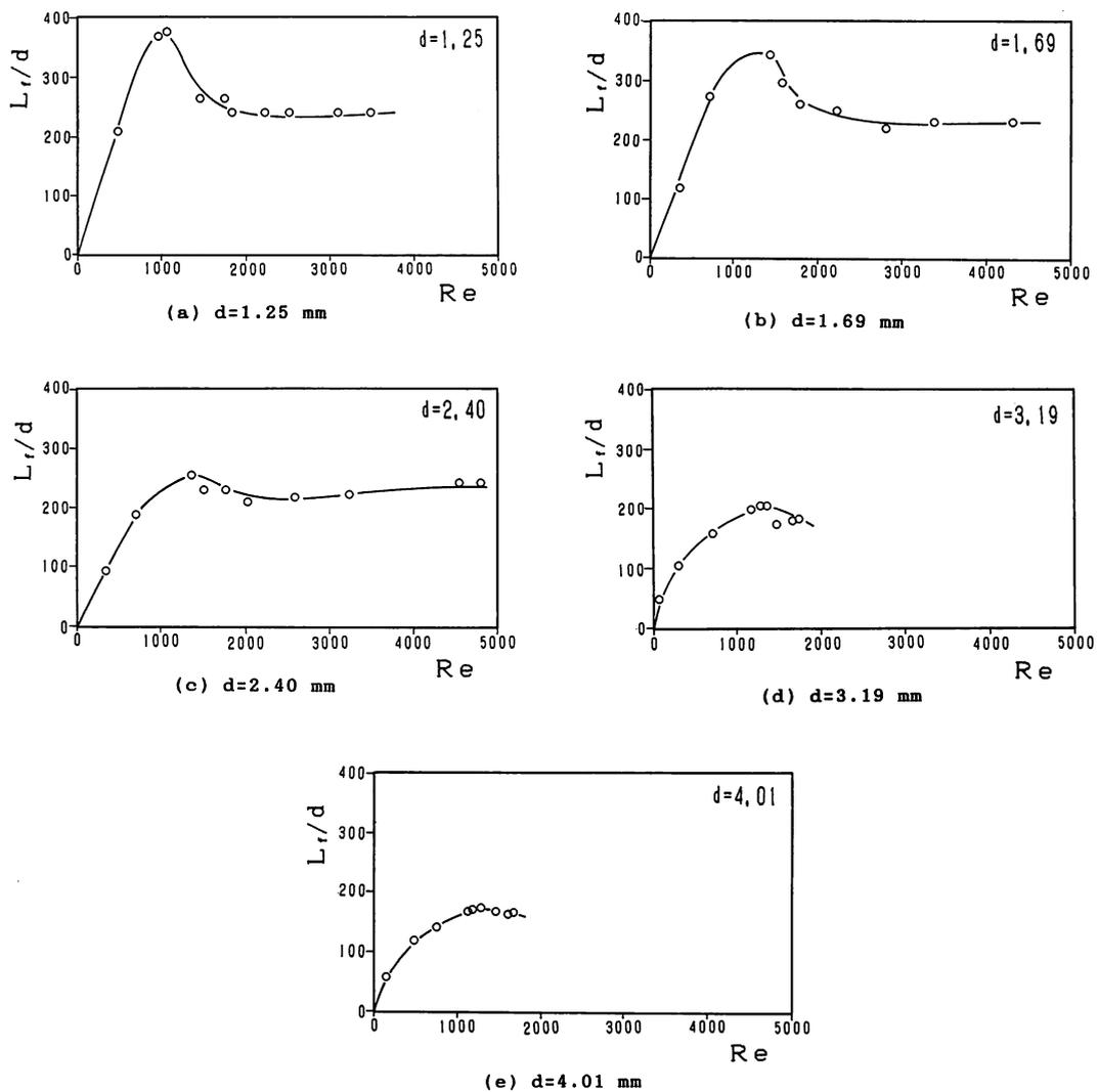
Fig. 5 Comparison of the flame lengths for different nozzle sizes
