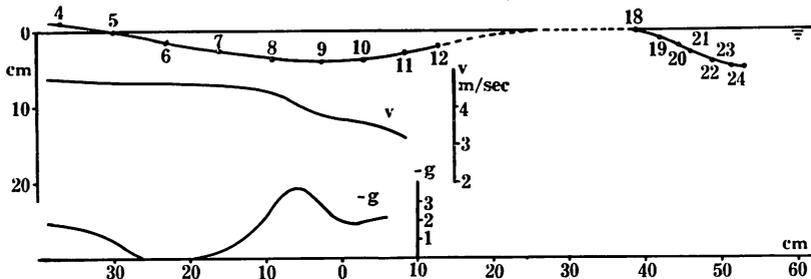
Fig. 8. Path of a projectile in the air and in the water, its velocity and acceleration.
