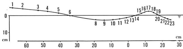
Fig. 4-2. Path of the projectile in the air and in the water
