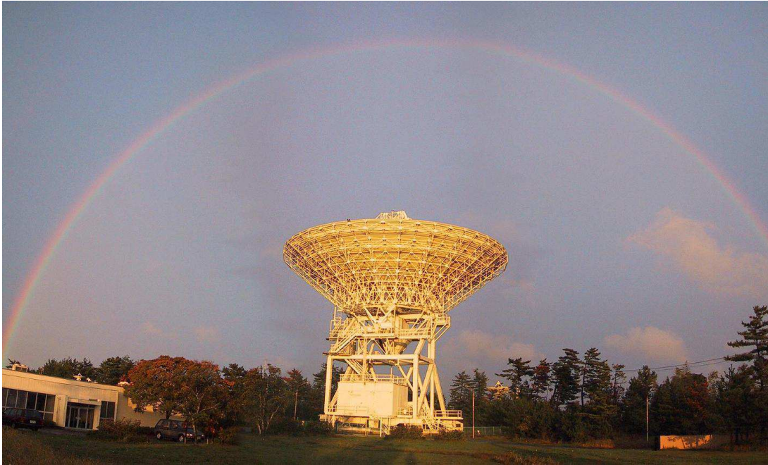
Figure 6.3: 34 m NICT Kashima radio telescope - Image of the 34 m NICT Kashima radio telescope used for the \text{NH}_3 mapping observations.
