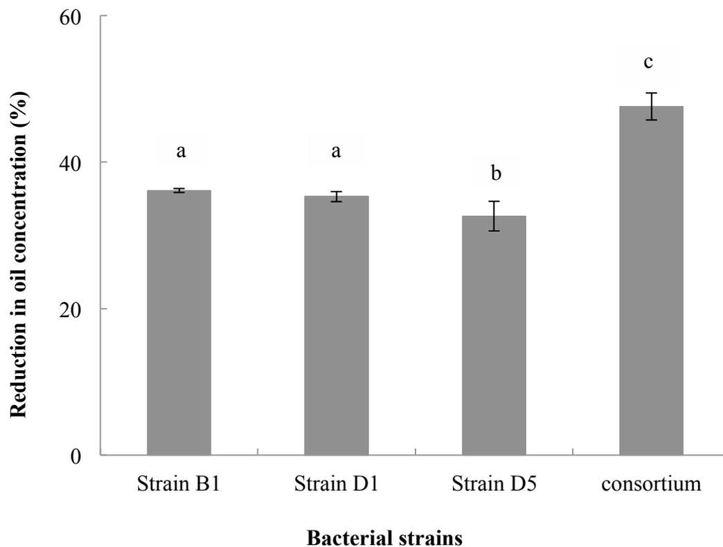
Fig. 1-3. Gravimetric determination of residual heavy oil in the BHMS media to which the bacterial strains or their consortium were added as a free-living form. The values represent the mean of three replicates after 30 days of incubation. The error bars show the standard deviation. The letter above each bar indicates a significant difference at  $p < 0.05$ .
