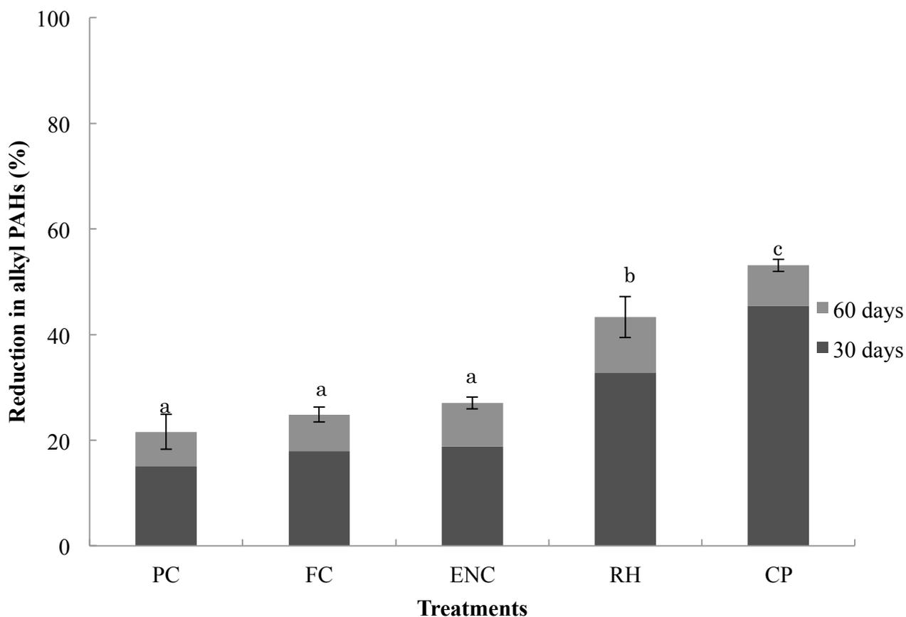
FIG. 2-5. Reduction in total alkyl polycyclic aromatic hydrocarbons in the different microcosms relative to abiotic control after 30- and 60-days incubation. Values represent the mean of three replicates. Error bars show the standard deviation. Different letters above the bars indicate significant difference at  $p < 0.05$ . Abbreviations of the treatments are shown in Table 2-2.
