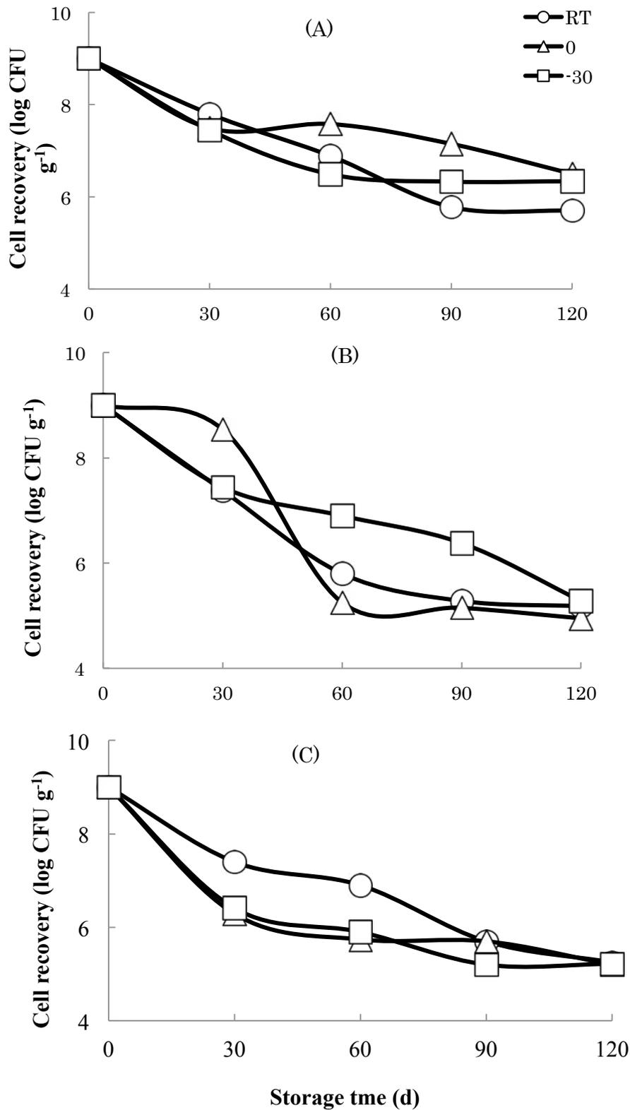
FIG. 2-7. Time course of the changes in viable counts obtained from the immobilized consortia (A, rice hull; B, cocopeat; C, encapsulated) stored in different temperatures, room temperature (open circles), 0°C (open triangles), and -30°C (open squares).
