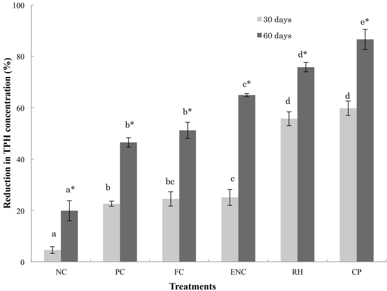
FIG. 2-2. Gravimetric determination of reduction in total petroleum hydrocarbon concentration of different seawater microcosms after 30 and 60 days of incubation. Values represent mean of three replicates. Error bars show the standard deviation. Different letters above the bars indicate significant difference at  $p < 0.05$ . Significant differences of day 60 measurements are indicated by letter with asterisk (\*) above the bars. Abbreviations of the treatments are shown in Table 2-2.
