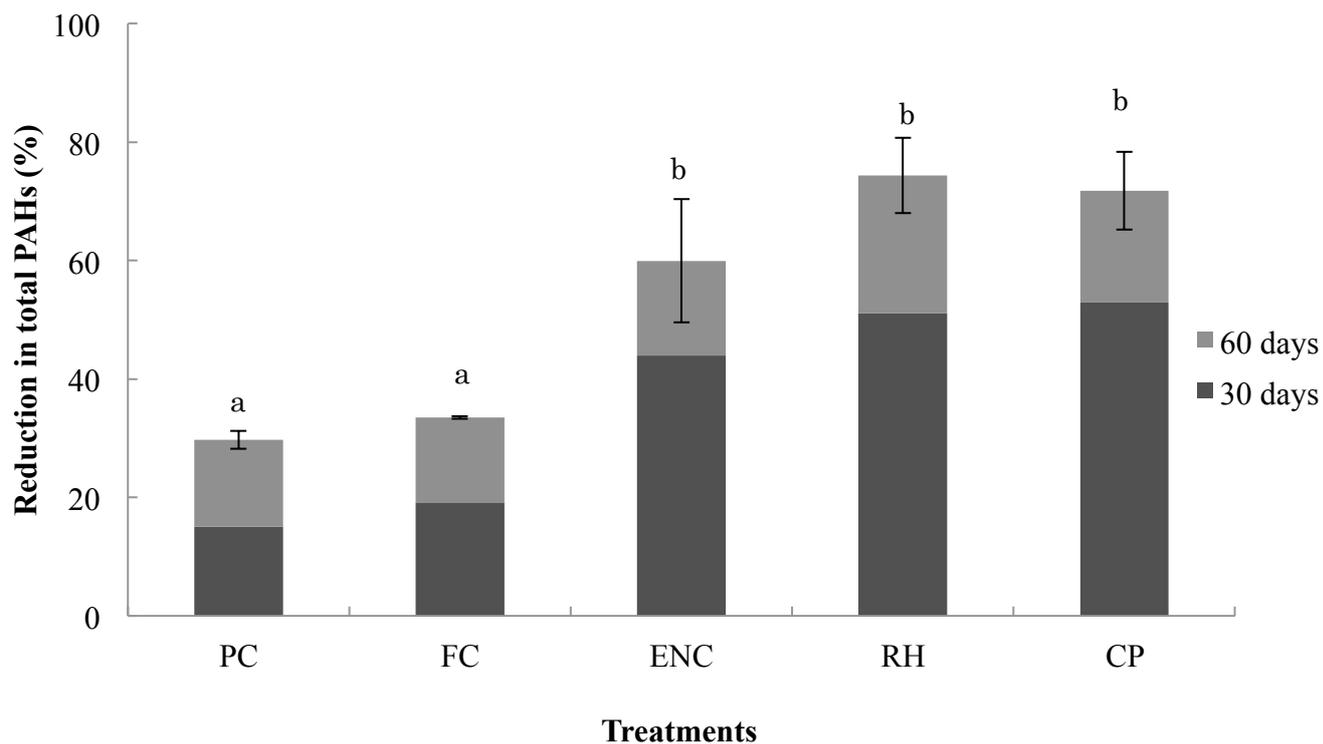
FIG. 2-4. Reduction in total polycyclic aromatic hydrocarbons in the different microcosms relative to abiotic control (NC) after 30- and 60-days incubation. Values represent the mean of three replicates. Error bars show the standard deviation. Different letters above the bars indicate significant difference at  $p < 0.05$ . The treatments indicated by the abbreviated names are shown in Table 2-2.
