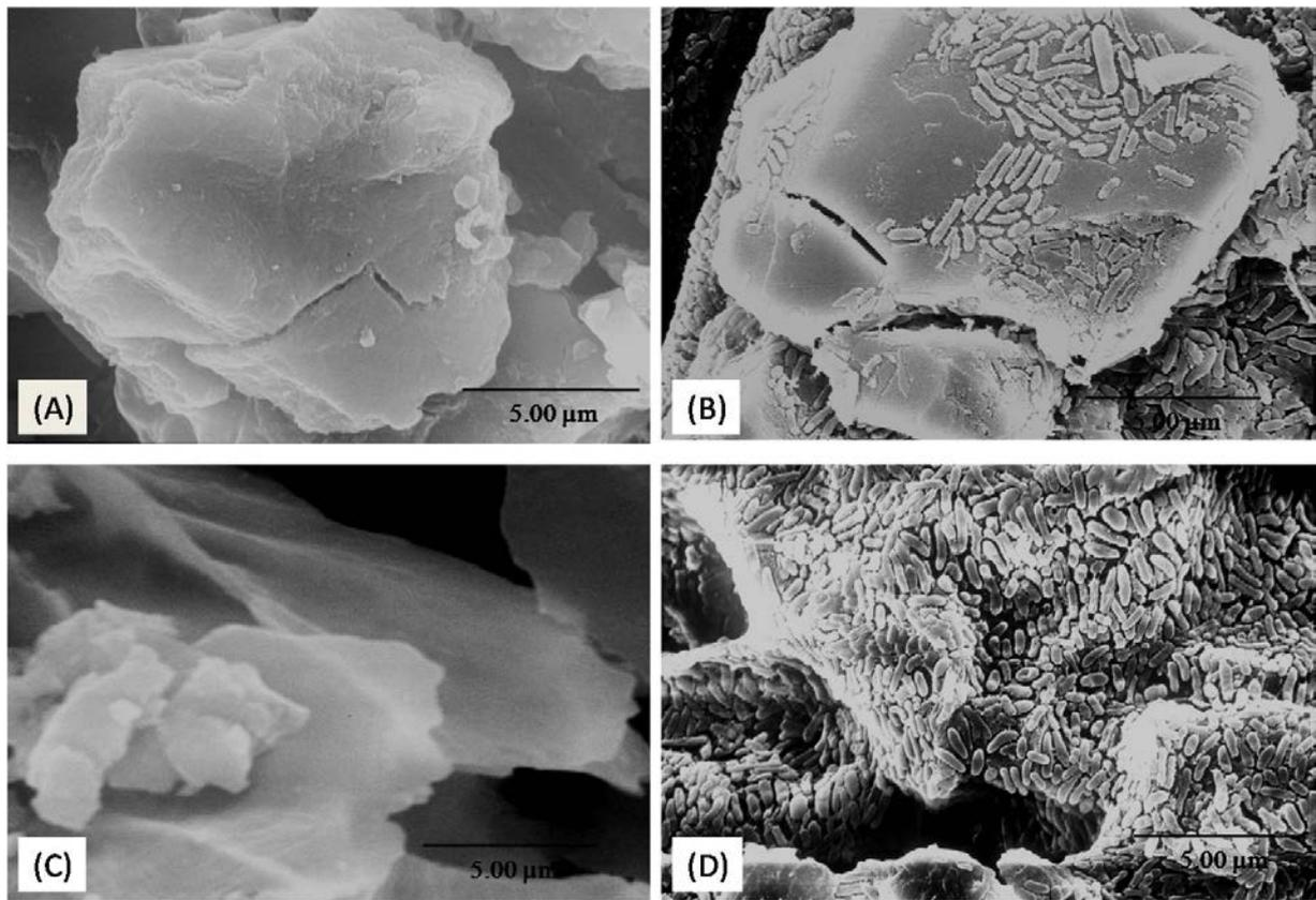
FIG. 2-1. Scanning electron microscopic images of the biocarriers without the bacteria (A, rice hull powder; C, cocopeat) and the consortium colonizing the surface of the biocarriers (B, rice hull powder; D, cocopeat).
