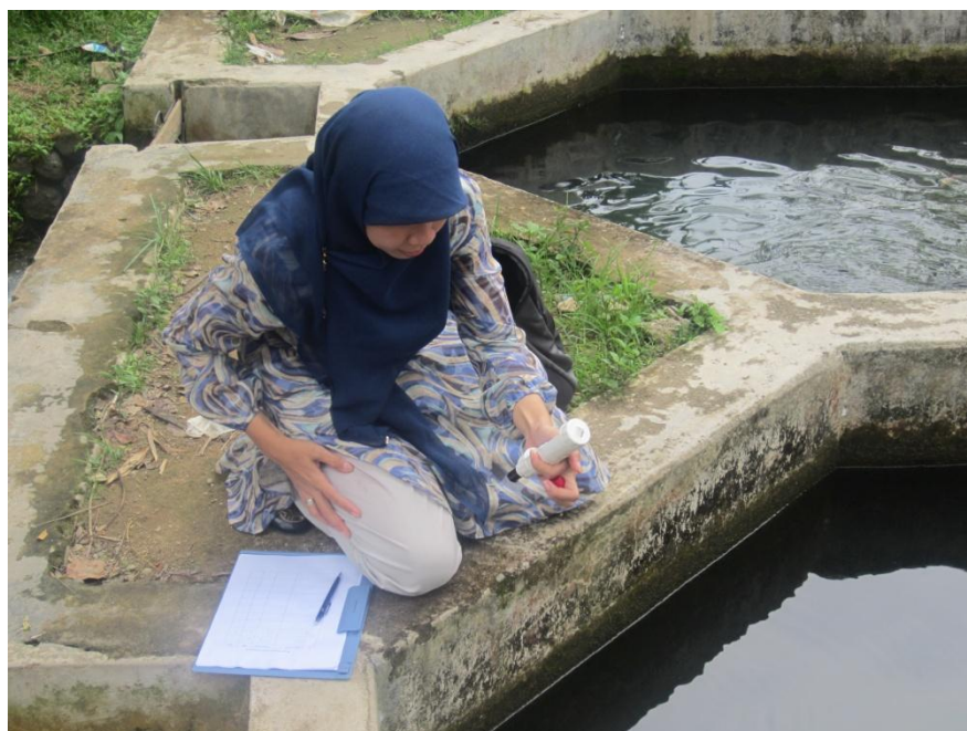
Figure 3.1 DO measurements in pond
