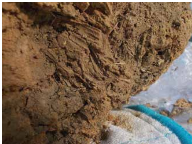
Fig. 70: Traces of organic matter used as temper.
