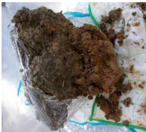
Fig. 69: The sample at the beginning of the exposure process. Separation of the darker inner layers (left) and the lighter outer layers (right).
