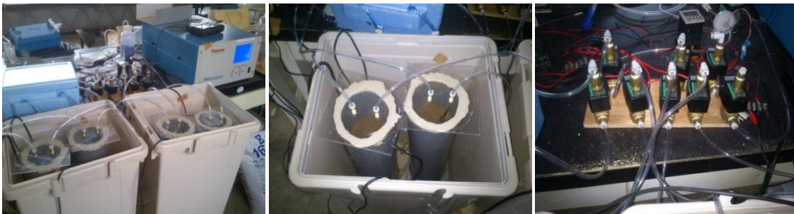
Figure 155: Closed chamber system installed. a) Upper right, the Thermo Scientific Analyzer 46i; installed cylinders in the foreground; b) Installation of soil moisture sensor (EC-5) and temperature sensor (5TE); c) Solenoid valves attached to inflows and outflows of each cylinder.
