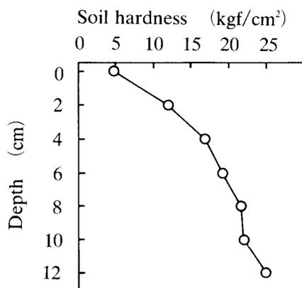
Fig. 2. Soil hardness of the tested field.
