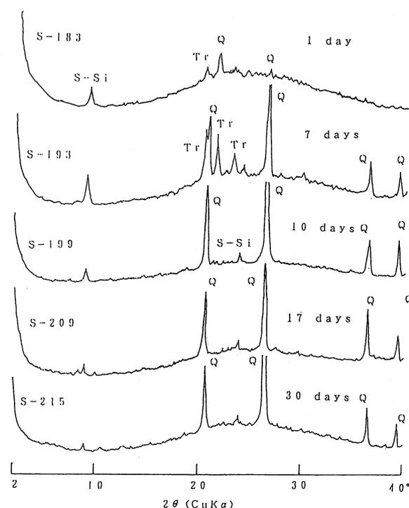
Fig. 7. X-ray powder diffraction patterns of the mixture of amorphous silica (3g) and NaOH (0.3g) after heating at 800°C for various time.
