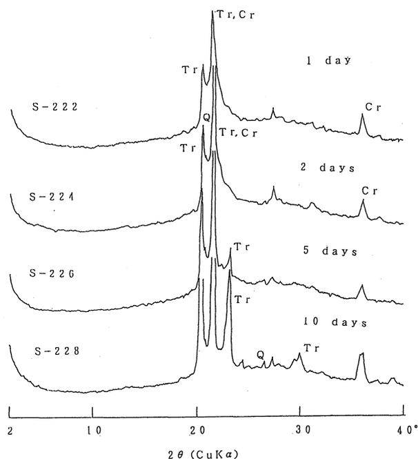
Fig. 11. X-ray powder diffraction patterns of the mixture of amorphous silica (2g) and KOH (0.1g) after heating at 800°C for various time.
