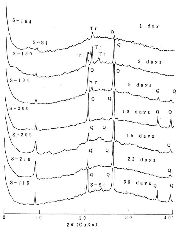
Fig. 8. X-ray powder diffraction patterns of the mixture of amorphous silica (3g) and NaOH (1g) after heating at 800°C for various time.
