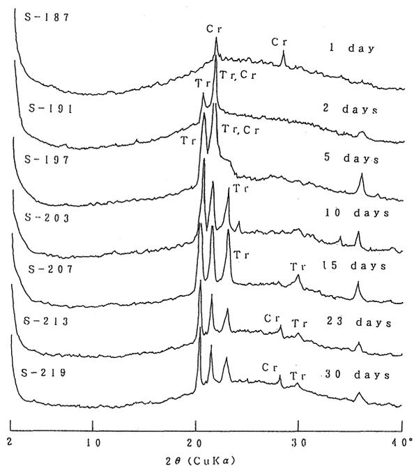
Fig. 13. X-ray powder diffraction patterns of the mixture of amorphous silica (3g) and KOH (1g) after heating at 800°C for various time.
