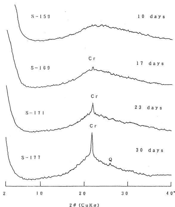
Fig. 1. X-ray powder diffraction patterns of the mixture of amorphous silica (3g) and  $\text{Na}_2\text{SO}_4$  (0.3g) after heating at  $800^\circ\text{C}$  for various time.
