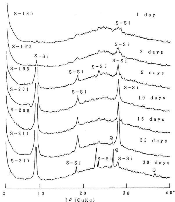
Fig. 9. X-ray powder diffraction patterns of the mixture of amorphous silica (1.5g) and NaOH (1.5g) after heating at 800°C for various time.
