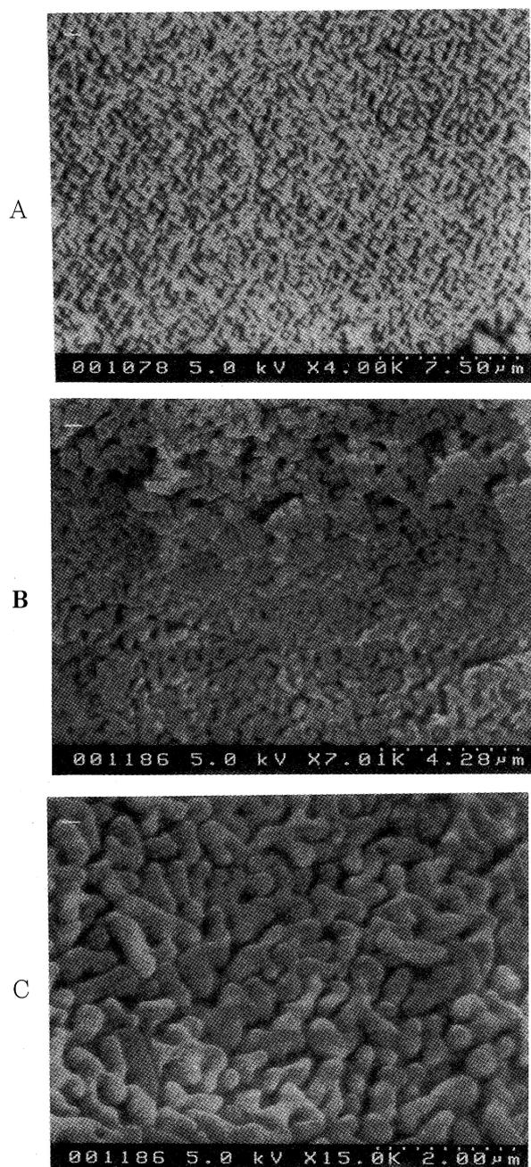
Fig. 3. Scanning electron micrographs of the products from the mixtures of amorphous silica and  $\text{Na}_2\text{SO}_4$  after for 30 days.
