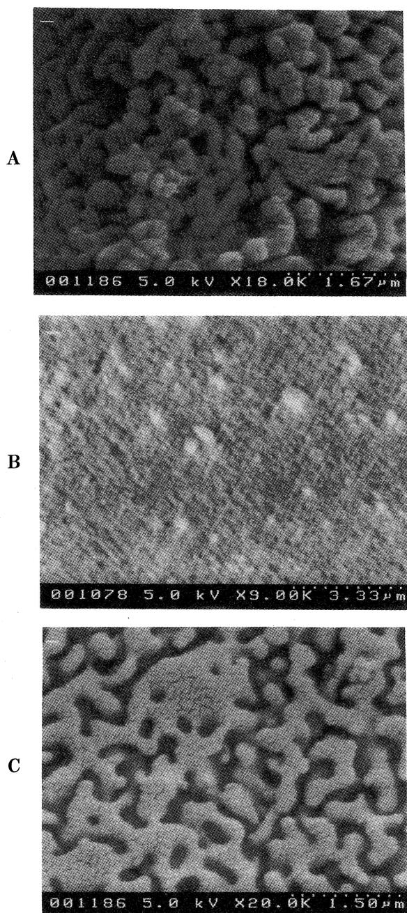
Fig. 5. Scanning electron micrographs of the products from the mixtures of amorphous silica and  $K_2SO_4$  after for 30 days.
