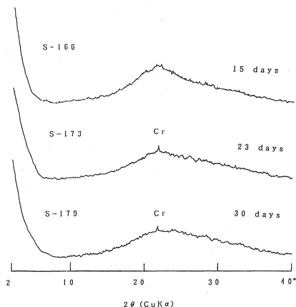
Fig. 2. X-ray powder diffraction patterns of the mixture of amorphous silica (1.5g) and  $\text{Na}_2\text{SO}_4$  (1.5g) after heating at  $800^\circ\text{C}$  for various time.
