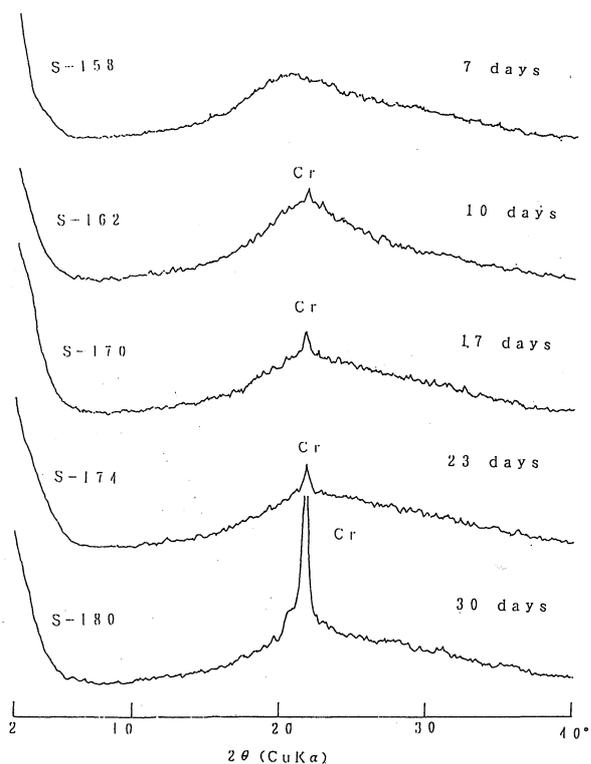
Fig. 4. X-ray powder diffraction patterns of the mixture of amorphous silica (3g) and  $K_2SO_4$  (0.3g) after heating at 800 °C for various time.
