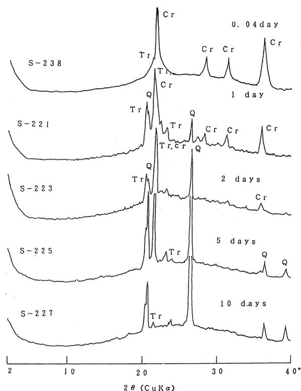
Fig. 6. X-ray powder diffraction patterns of the mixture of amorphous silica (2g) and NaOH (0.1g) after heating for various time.
