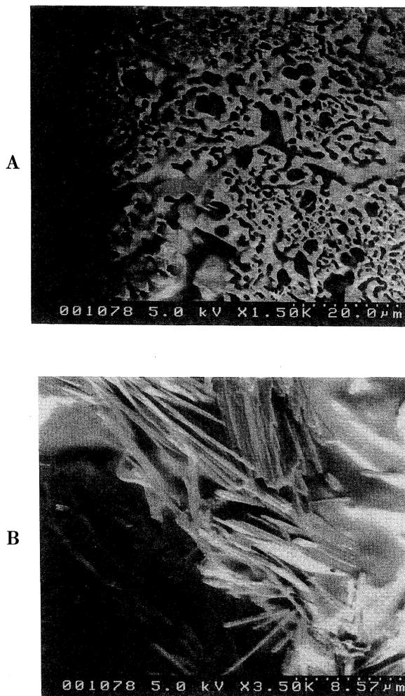
Fig. 10. Scanning electron micrographs of the products from the mixtures of amorphous silica and NaOH after for 30 days.
