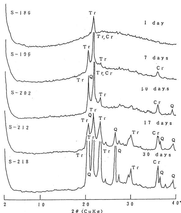
Fig. 12. X-ray powder diffraction patterns of the mixture of amorphous silica (3g) and KOH (0.3g) after heating at 800°C for various time.
