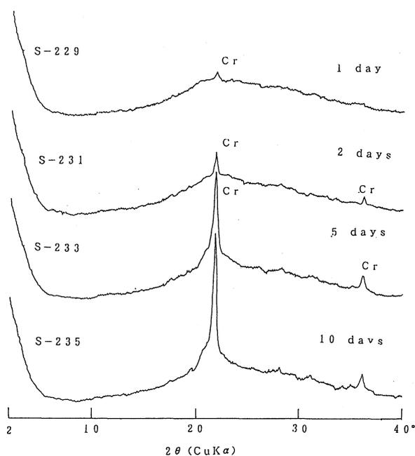
Fig. 15. X-ray powder diffraction patterns of the mixture of amorphous silica (2g) and NaOH (0.1g) after heating at 600°C for various time.
