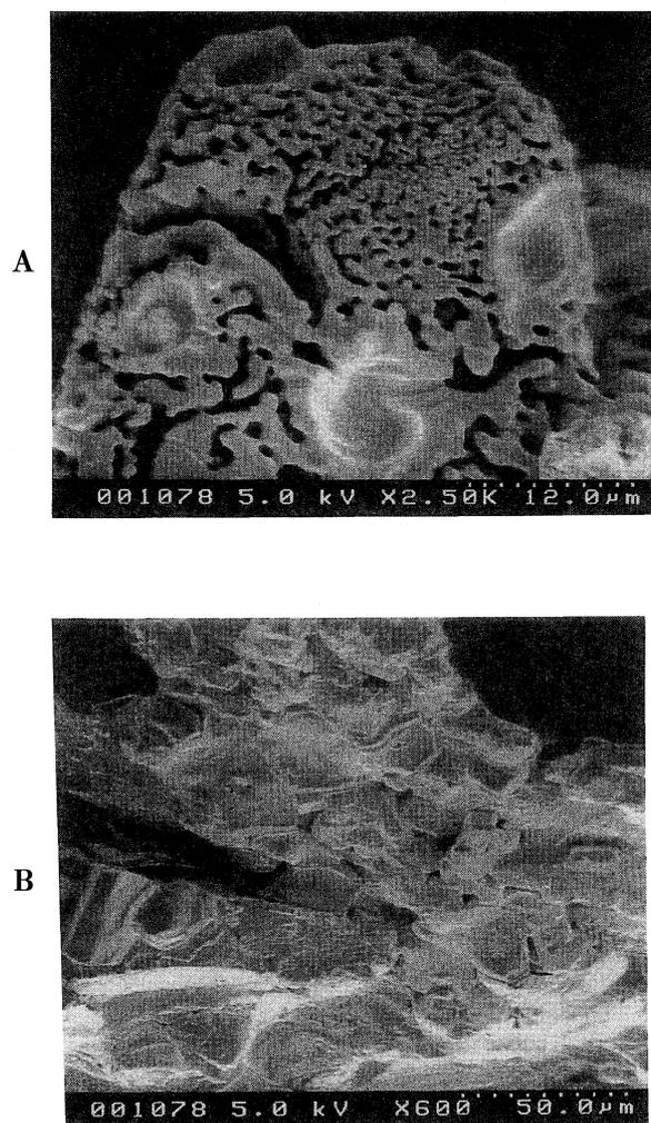
Fig. 14. Scanning electron micrographs of the products from the mixtures of amorphous silica and KOH after for 30 days.
