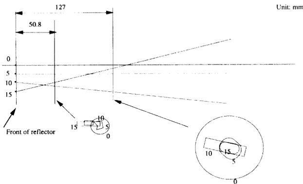
Fig. 8 Ray tracing estimated from patterns of measurement planes for an actual reflector lamp
