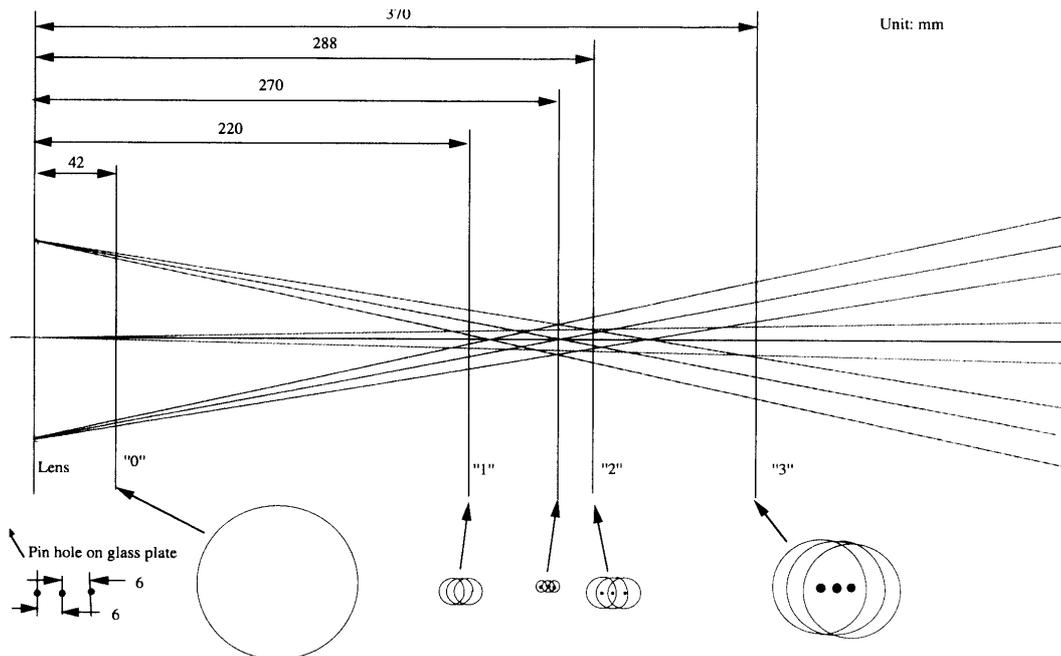
Fig. 6 Ray tracing estimated from the patterns on the measurement planes
