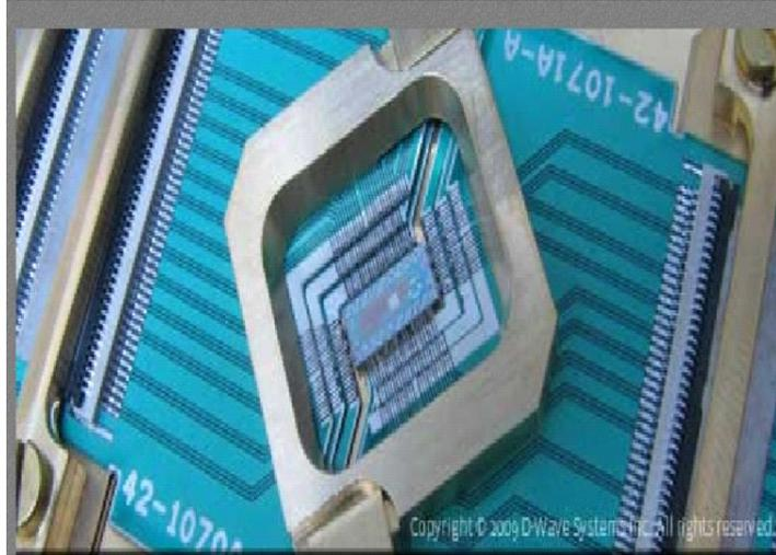
Figure 2.1: First Quantum CPU with 128 qubits, designed and presented by D-Wave systems, February 2007. [12]
