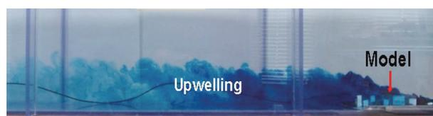
Fig.7 Image of upwelling induced by a marine structure model
