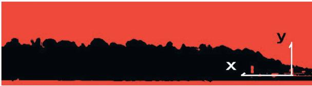
Fig.8 Binarized image of upwelling flow and coordinate system
