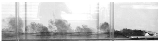
Fig.19 Image of upwelling induced by Mount(90) type structure
