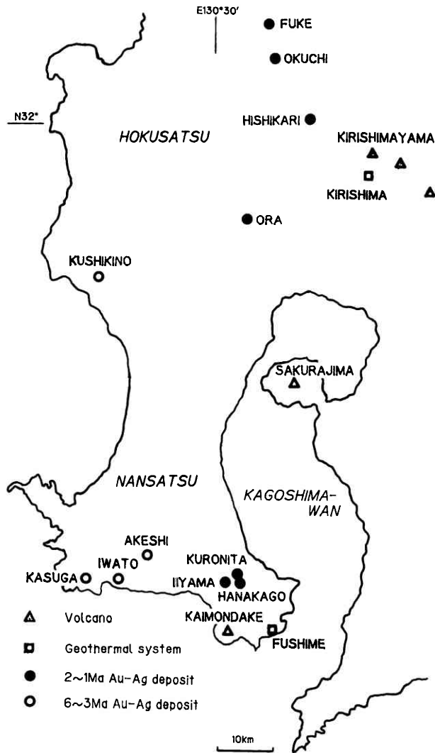
Fig. 1 K-Ar age for adularia or alunite from the gold-silver deposits (paleo-geothermal systems) in the Satsuma district, Kagoshima. Kushikino (串木野) : 4.0 \pm 0.3 \text{ Ma}^1 . Kasuga (春日) : 5.5 \pm 0.4 \text{ Ma}^2 . Iwato (岩戸) : 4.7 \pm 1.0 \text{ Ma}^2 , 4.4 \pm 0.7 \text{ Ma}^2 , 4.13 \pm 0.78 \text{ Ma}^3 . Akeshi (赤石) : 3.7 \pm 1.1 \text{ Ma}^2 . Fuke (布計) : 1.40 \pm 0.19 \text{ Ma}^4 . Okuchi (大口) : 1.1 \pm 0.5 \text{ Ma}^4 . Hishikari (菱刈) : 1.5 \pm 0.3 \text{ Ma}^5 , 0.98 \pm 0.04 \text{ Ma}^6 , 0.97 \pm 0.04 \text{ Ma}^6 , 0.86 \pm 0.12 \text{ Ma}^4 . Ora (大良) : 1.8 \pm 0.2 \text{ Ma}^5 . Iiyama (飯山) : 1.5 \pm 0.1 \text{ Ma}^7 . Kuronita (黒仁田) : 1.3 \pm 0.7 \text{ Ma}^4 . Hanakago (花籠) : 1.1 \pm 0.5 \text{ Ma}^8 .
