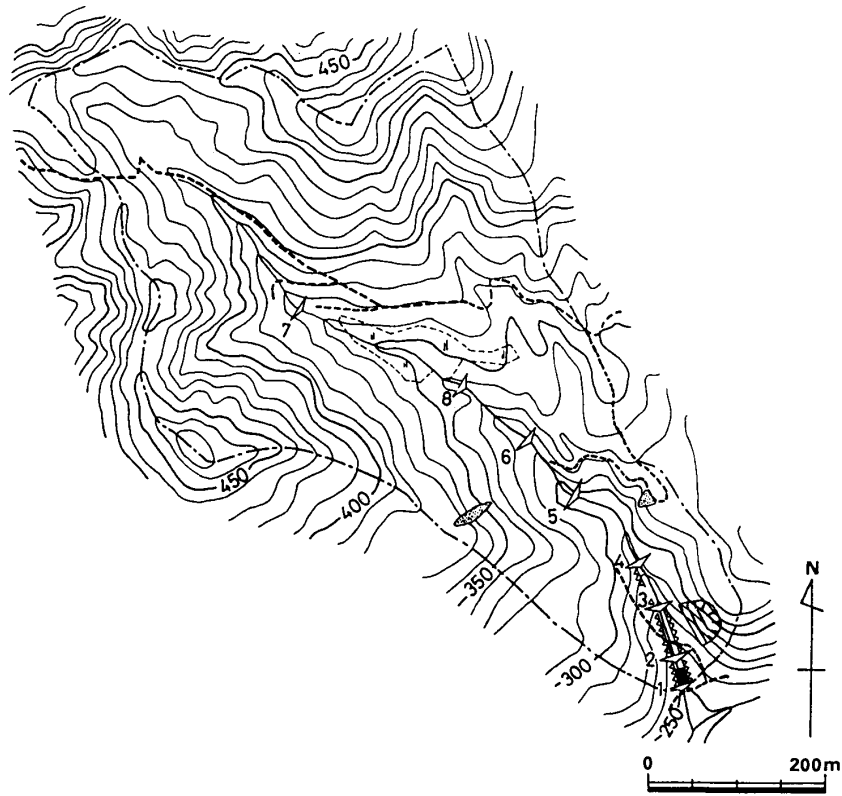
Fig. 3.14 Topography of Kooriyama experimental catchment. ■ : Gauging weir and rain gauge
