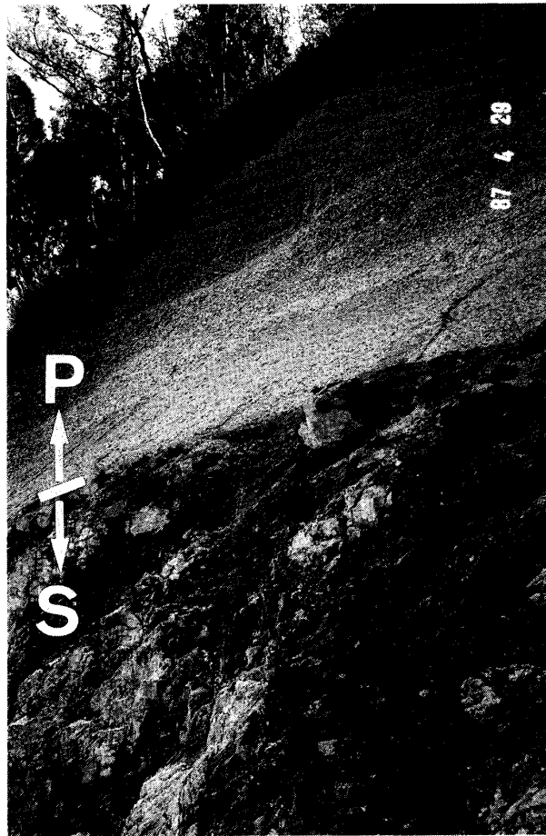
Photo. 3.2 Typical geological profile in No.2 Takakuma experimental catchment. S: Sandstone (Shimanto group), P: Pyroclastic fall
