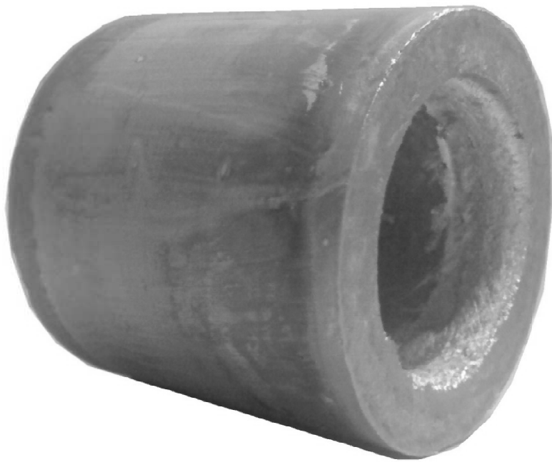
Fig. 2-4 Appearance of FGM thick-walled tube.
