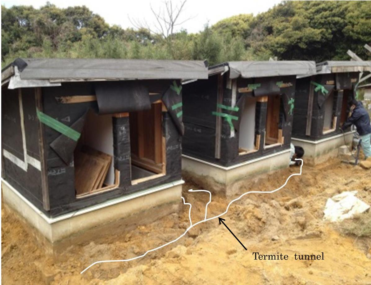
Fig.1-7. The termite tunnel for bait
