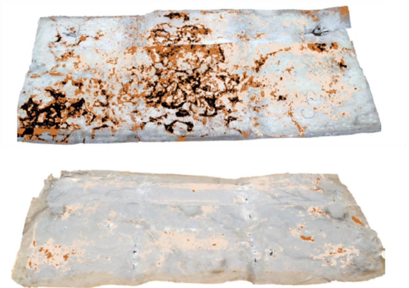
Fig.1-12. The adhesion of termite soil on the underside surface of the PE-sheets
