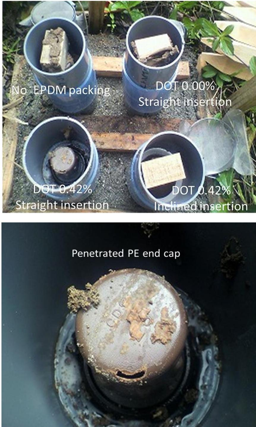
Fig.2-15. Condition of EPDM packing for supply piping after field experiment
