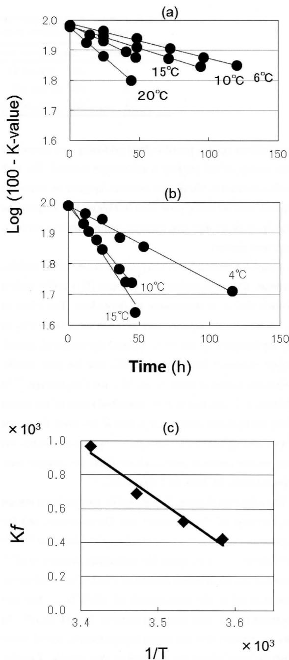
Fig. 5 Effects of temperatures on rate constant of freshness-lowering in big-eyed tuna (a) and bonito (b). Arrhenius' plot (c) was obtained from the rate constant of big-eyed tuna.
