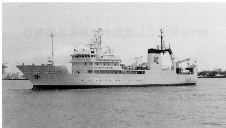
Plate 1. The training ship Kagoshima Maru. (1284GT, Length/66.92M, Breadth/12.1M, Depth/4.5M, Capacity/ 72persons)
