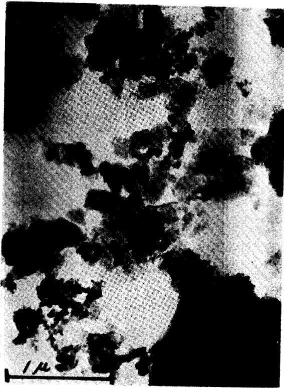
Fig. 3-1. Electron micrograph of Ca-clay ( <2\mu ) from topsoil of paddy field of volcanic ash soil, sample No. 1
