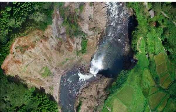
Photo18. Debris by major slope failure once made a natural dam, then flushed by the river flow
