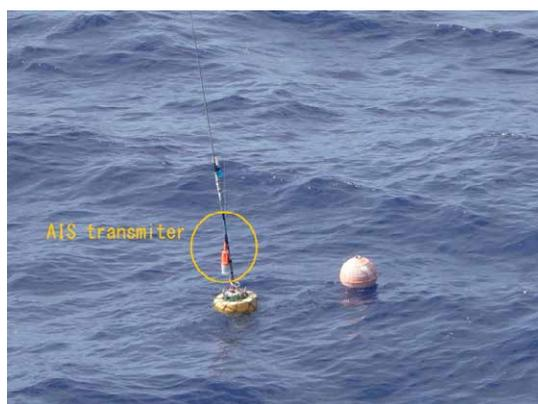
Plate 2. Longline float and radio buoy with AIS
