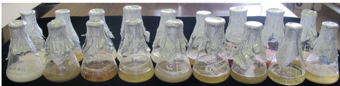
Fig.III.1. Fermented Pikovskaya broth culture for organic acid determination by HPLC inoculated with 16 phosphate solubilizing fungal strains.
