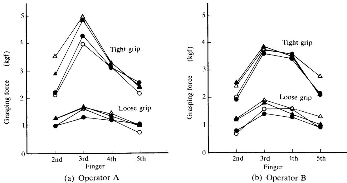
Fig. 3. Measured grasping forces on each finger at tight and loose grip.
