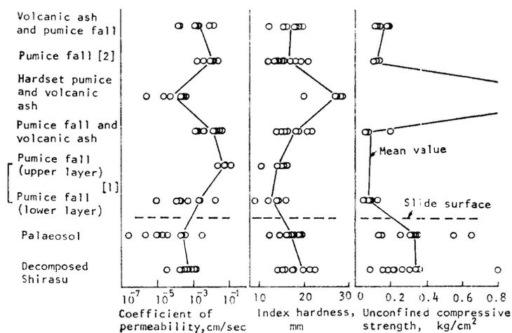
Fig. 10. Geotechnical properties of the Shirasu, and the pumice and volcanic ash beds.
