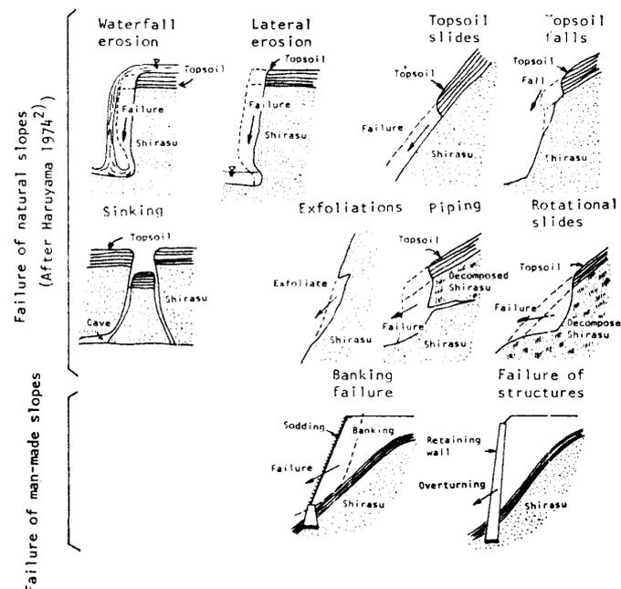
Fig. 3. Basic types of slope-failures in the Shirasu region.
