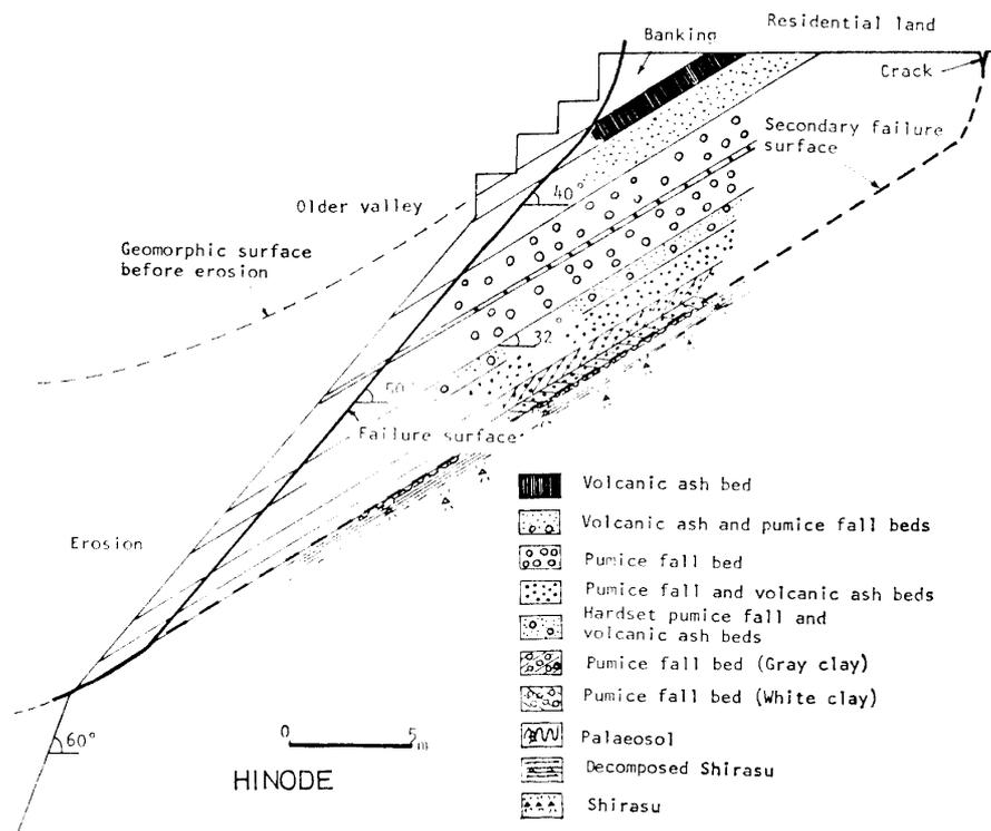
Fig. 4. A typical example of topsoil slides at Hinode, Kagoshima-shi.
