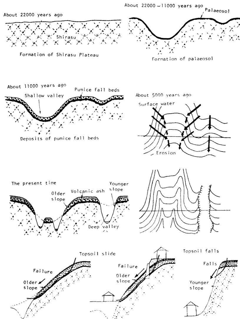
Fig. 6. Schematic topographic evolution process of the Shirasu plateau and forms of the slope-failures (This figure was made based on Iwamatsu 1976<sup>3)</sup>).
