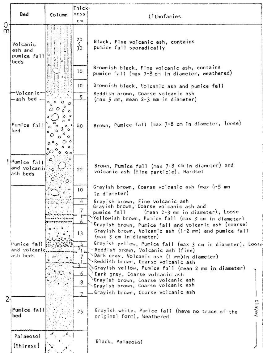
Fig. 9. A typical example of the geologic columnar section.
