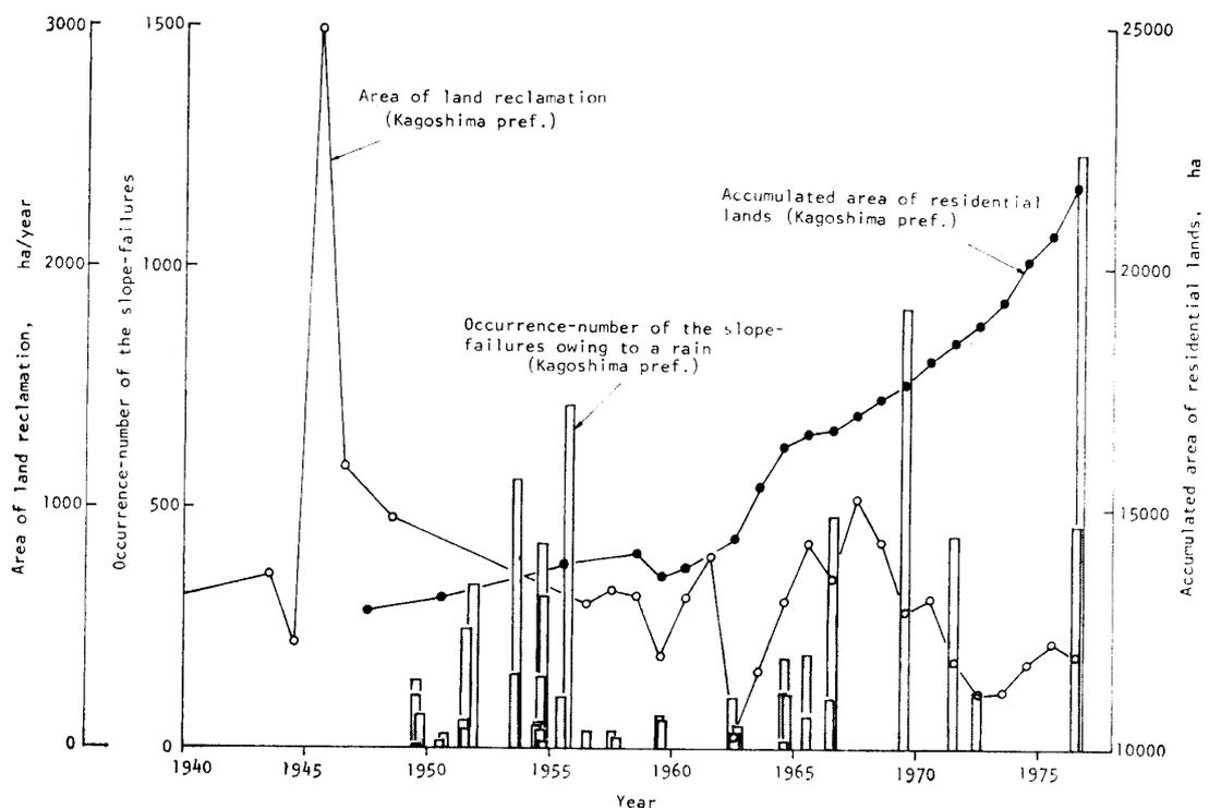
Fig. 2. Transitions of occurrence-number of the slope-failures owing to a rain, area of land reclamation during a year and accumulated area of residential lands.
