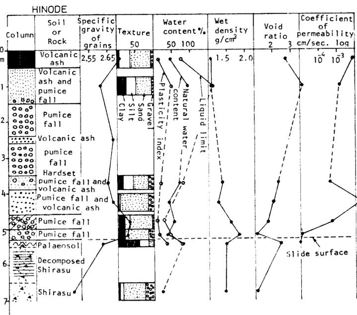
Fig. 5. Geotechnical properties of the Shirasu ground at Hinode, Kagoshima-shi.
