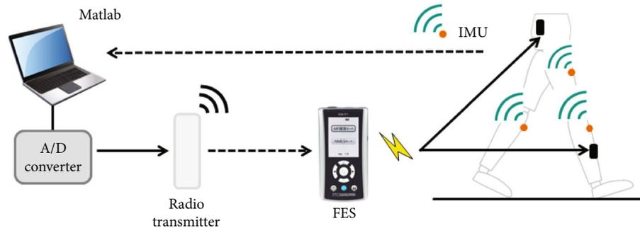
FIGURE 1: Schematic diagram of functional electrical stimulation (FES) control. The solid line represents wired processing, and the broken line represents wireless processing. The FES was held by the patient. Orange dots mark the position of the magnetic inertial measurement units (IMU).
