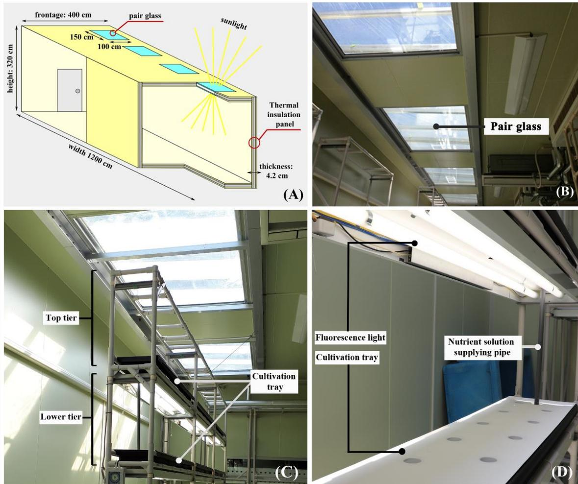
**Fig. 3.2.** Solar plant factory diagram (A), revised rooftop with pair glasses (B), vertical cultivation shelves with the top tier (S, sunlight) and the lower tier (SA, low sunlight and artificial light) (C), and cultivation tray (D).
