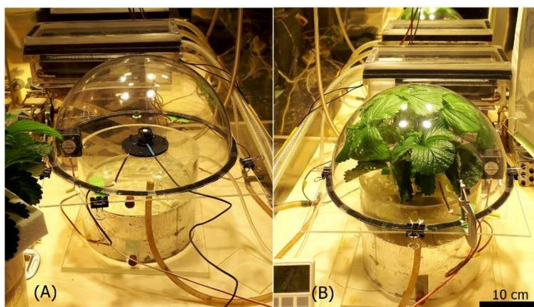
**Fig. 2.3** Assimilation chamber without plant (A) and with plant (B) used for the whole-plant method (Wp method) to measure the whole-plant diurnal photosynthesis and whole-plant light response curve.
