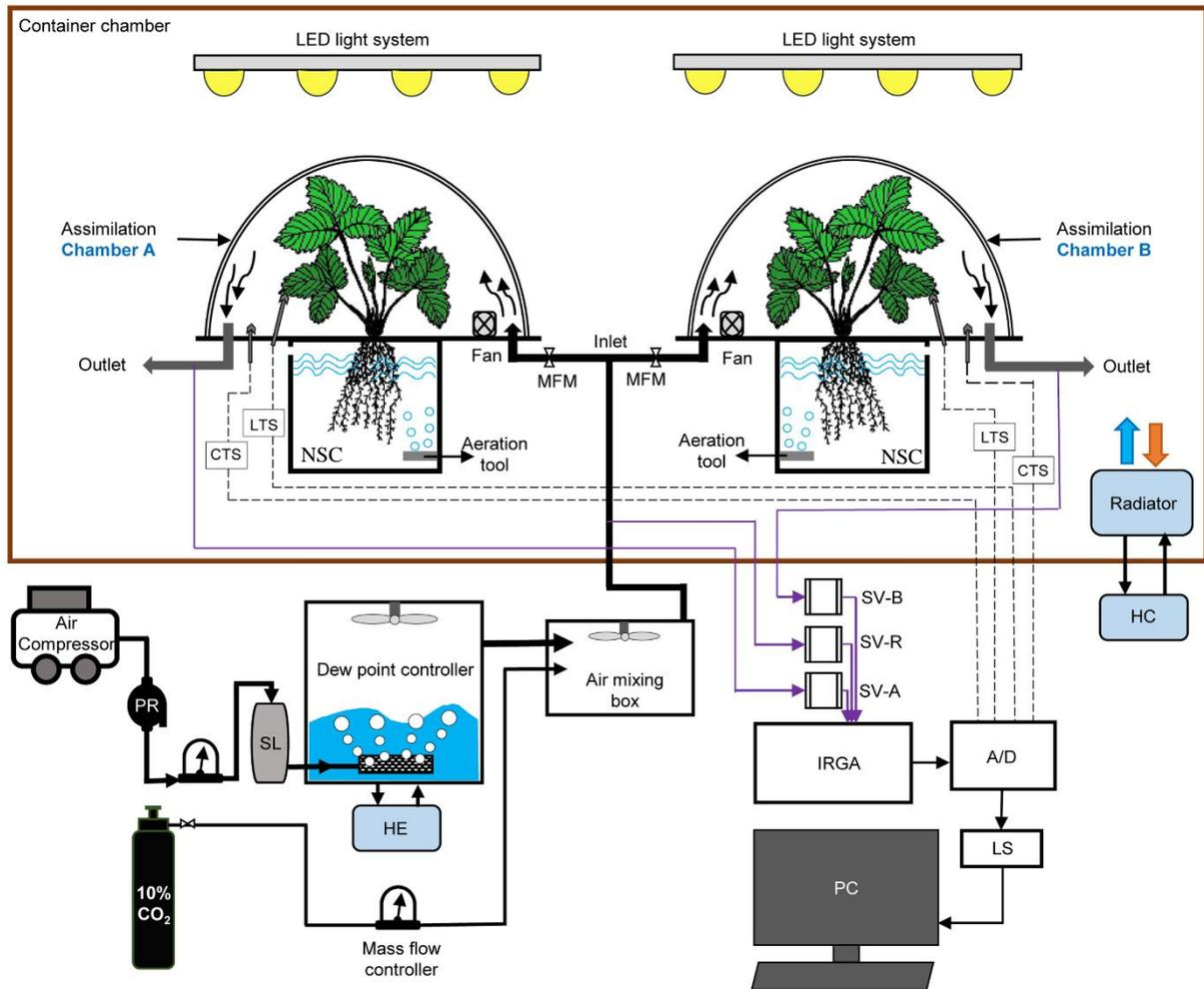
**Fig. 2.2** Schematic diagram of photosynthetic close-chamber measurement system used for strawberry plant.
