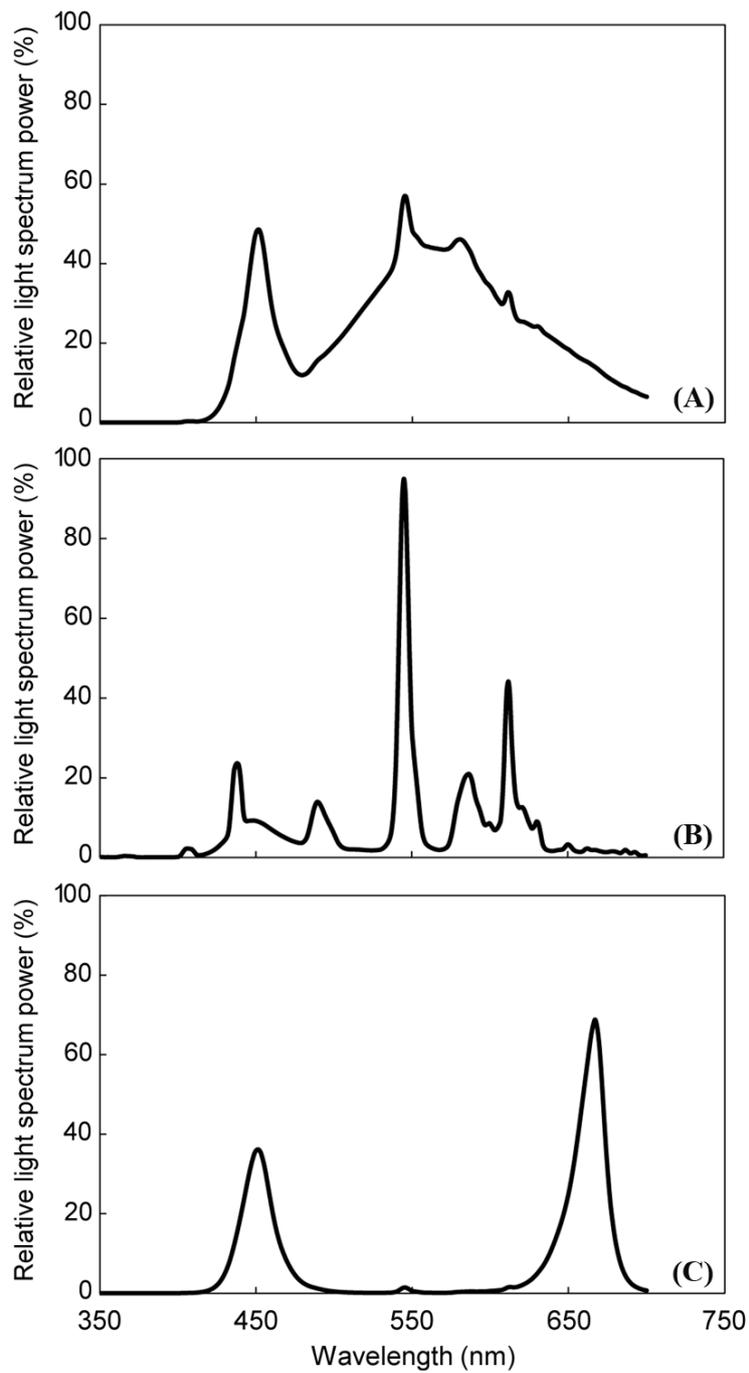
**Fig. 4.1.** The spectral photon distribution of (A) white LED light (WL), (B) white fluorescence light (WF), and (C) purple LED light (PL).
