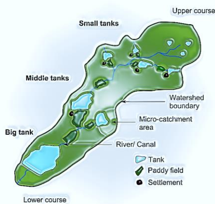
Schematic view of a cascaded tank-village system (Schütt, Bebermeier, & Meister, 2013)
