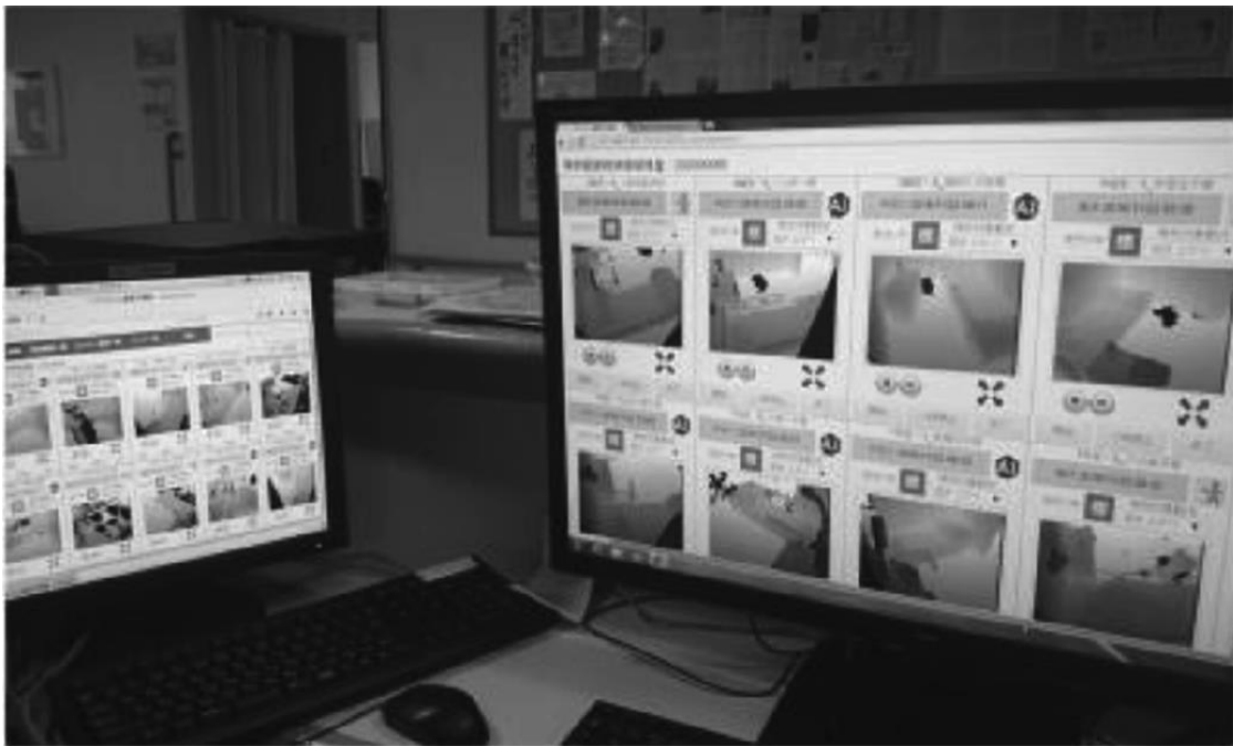
Figure 12: Monitoring System of Care Recipients's Movement by an Infra-red Radiation Camera [38]
