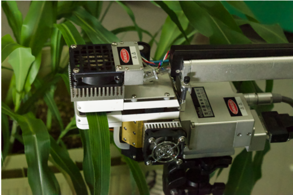
Figure 4-2. Gas exchange measurement by using a portable gas exchange measurement system (LI-6400, Li-Cor Inc., Lincoln, NE, USA) equipped with the standard leaf chamber (chamber area of 6 cm 2 ).
