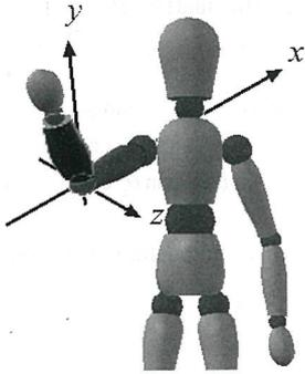
Figure 3. Child–parent relationship. The endpoint of the child segment of right forearm is defined in a local frame of reference set to its parent of right shoulder.
