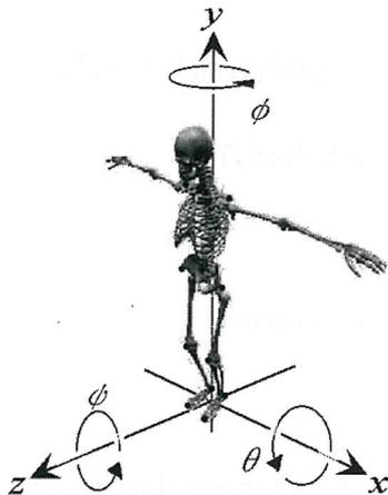
Figure 1. Base human model in the global frame of reference. Markers placed on individual joints are shown as dots in the Figure. The direction of rotation follows the right hand rule, as indicated as rings around axes.
