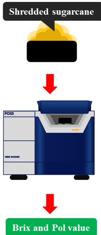
**Figure 1.5:** Diagram of using benchtop Vis-NIR spectrometer in sugar mill
