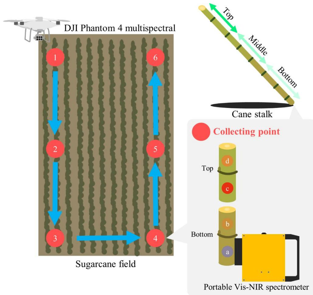
**Figure 3.5:** Example of the flight contour and details of using a portable Vis-NIR spectrometer to scan the sugarcane stalk twice on the bottom and top at the collection points.
