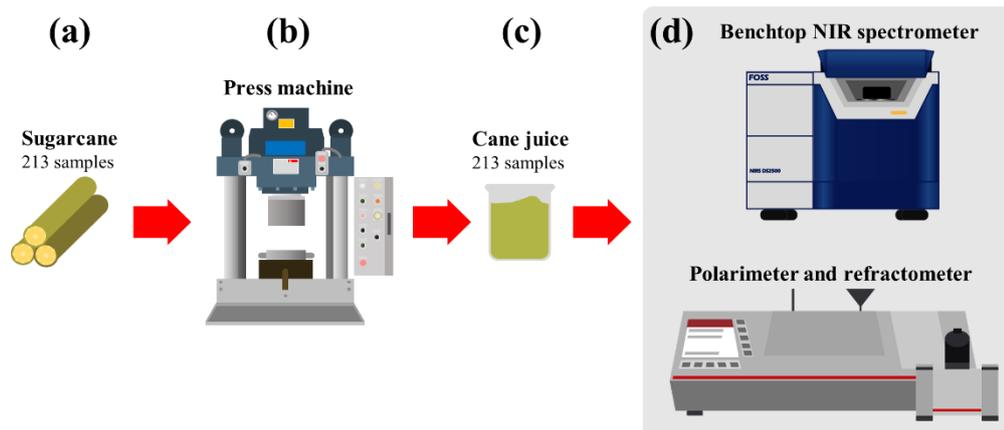
**Figure 3.2:** First experiment design outline: (a) Sugarcane billet samples were prepared by (b) pressing the stalks using a hydraulic press to extract (c) sugarcane juice to (d) measure Brix, Pol, and sugarcane spectra using a refractometer, polarimeter, and a benchtop Vis-NIR spectrometer.
