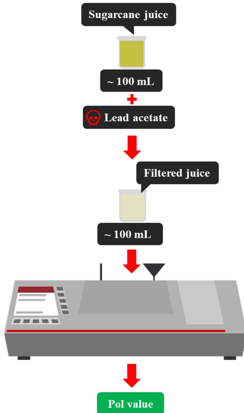
**Figure 1.4:** Diagram of present process to obtain sugarcane Pol value in sugar mill
