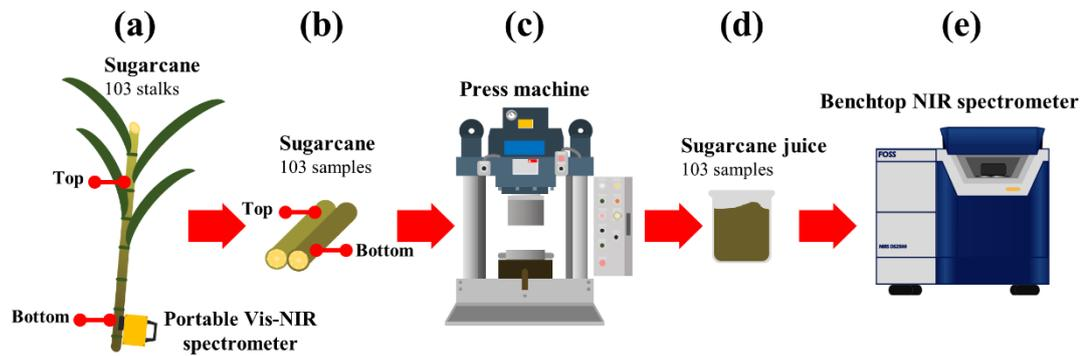
**Figure 3.3:** Second experiment design outline: (a) Scanning sugarcane stalk using a portable Vis-NIR spectrometer for sugarcane spectra. Then, (b) the sugarcane was harvested and prepared for (c) use in a hydraulic press to extract (c) sugarcane juice to (d) measure sugarcane spectra using a benchtop Vis-NIR spectrometer.
