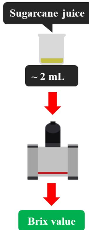
**Figure 1.3:** Diagram of present process to obtain sugarcane Brix value in sugar mill
