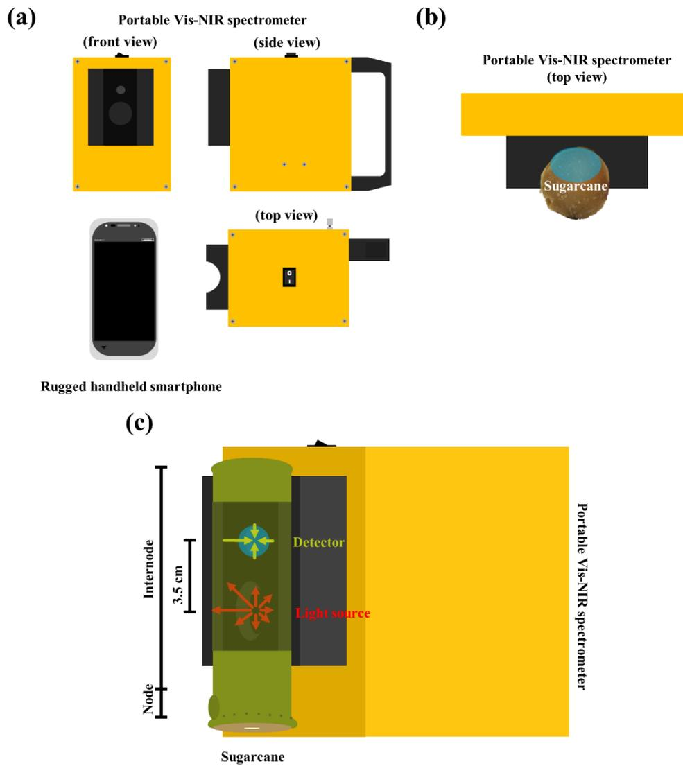
**Figure 3.4:** Portable NIR spectrometer. (b) Top view example of light transmission through sugarcane stalk. (c) An example of how a portable Vis-NIR spectrometer operates.
