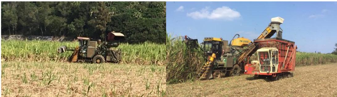
**Figure 2.3:** The sugarcane harvester small type (left) and large type (right)
