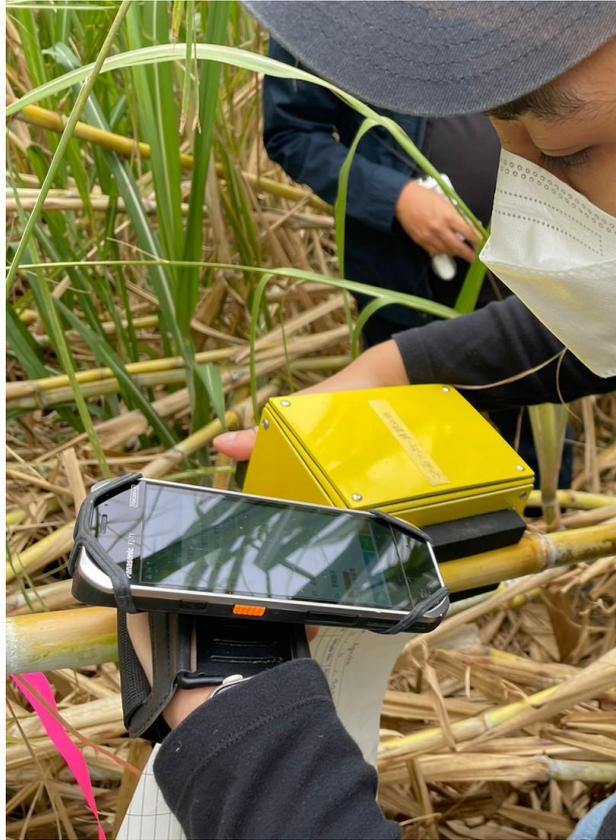
**Figure 3.6:** Photo of using a portable Vis-NIR spectrometer to scan the sugarcane stalk.
