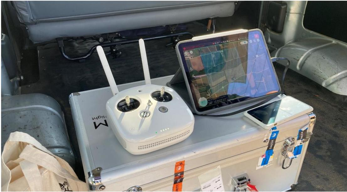
**Figure 3.8:** Photo of drone control using DJI GS Pro application.
