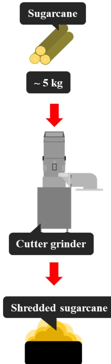
**Figure 1.6:** Diagram of process to obtain shredded sugarcane in sugar mill using cutter grinder
