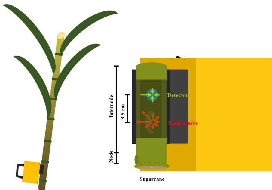
**Figure 1.8:** Example of demonstration of using a portable Vis-NIR spectrometer
