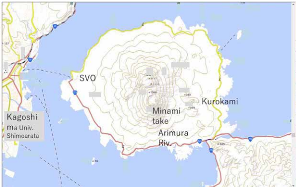
Fig.1. Sakurajima volcanic smoke observation radar configuration, Ku-RAD (Shimoarata), Solid State Marine Radar:SSR (SVO), SSR (Arimura Riv.), Marine Radar (Kurokami), Kashmir 3D.
