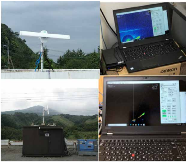
Fig.5. SVO antenna unit (upper left), SVO Control monitoring PC (upper right), Arimura Riv. antenna unit (lower left), Arimura Riv. Control monitoring PC (lower right)
