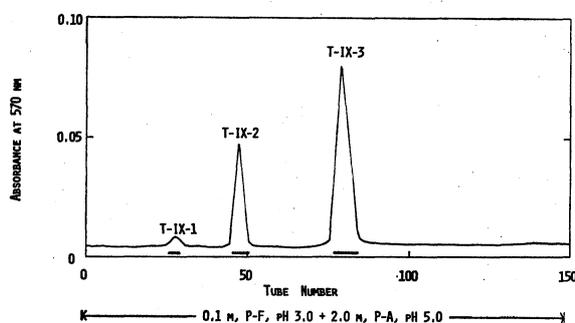
Fig. 8. Fractionation of CNBr-II-T-IX on a column ( $0.9 \times 50$ cm) of Dowex 50-X2. The chromatography was carried out at  $42^\circ$  at a flow rate of 25 ml per hour. Fractions of 2.5 ml were collected.
