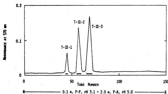
Fig. 19. Fractionation of CNBr-III-T-III on a column ( $0.9 \times 50$ cm) of Dowex 50-X2. The chromatography was carried out at  $42^\circ$  at a flow rate of 20 ml per hour. Fractions of 2.0 ml were collected.
