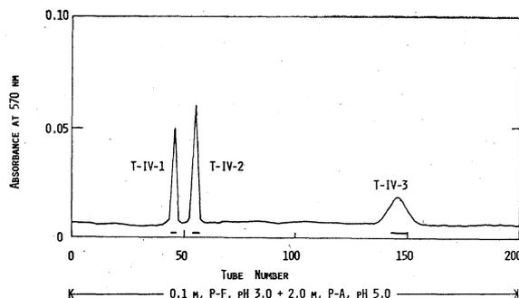
Fig. 6. Fractionation of CNBr-II-T-IV on a column ( $0.9 \times 50$ cm) of Dowex 50-X2. The chromatography was carried out at  $42^\circ$  at a flow rate of 20 ml per hour. The effluent was collected in 2.0 ml fractions.
