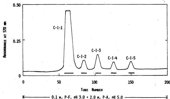
Fig. 12. Fractionation of CNBr-II-C-I on a column (0.9×50cm) of Dowex 50-X2. The chromatography was carried out at 28° at a flow rate of 25 ml per hour. Fractions of 2.5 ml were collected.
