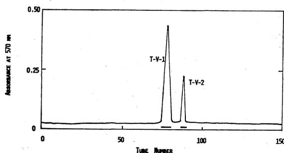
Fig. 20. Gel filtration of CNBr-III-T-V on a column ( $1.0 \times 100$ cm) of Bio-Gel P-10. The details are described in the Fig. 10.
