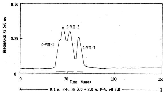
Fig. 14. Fractionation of CNBr-II-C-VIII on a column ( $0.9 \times 50$ cm) of Dowex 50-X2. The chromatography was carried out at  $40^\circ$  at a flow rate of 25 ml per hour. Fractions of 2.5 ml were collected.
