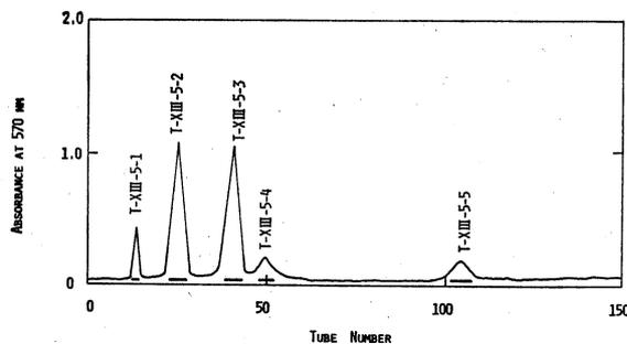
Fig. 10. Gel filtration of CNBr-II-T-XIII-5 on a column (1.3×105cm) of Bio-Gel P-10. The column was developed with 1.0 M formic acid at a flow rate of 20 ml per hour. Fractions of 2.0 ml were collected and monitored by ninhydrin method after alkaline hydrolysis.
