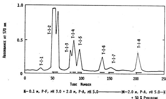
Fig. 4. Fractionation of CNBr-II-T-I on a column (0.9 × 50cm) of Dowex 50-X2. The chromatography was carried out at 42° at a flow rate of 25 ml per hour. Fractions of 2.5 ml were collected.
