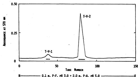
Fig. 7. Fractionation of CNBr-II-T-V on a column ( $0.9 \times 50$ cm) of Dowex 50-X2. The chromatography was carried out at  $42^\circ$  at a flow rate of 25 ml per hour. Fractions of 2.5 ml were collected.
