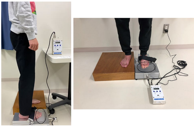
Fig.1 Measurement of toe pressure strength in standing position. Circles indicate force plates. In the standing position, the force plate should be adjusted so that only the toes ride on the force plate. Ankle joint is fixed with a belt, and force is applied to pressing on the floor with the toes
