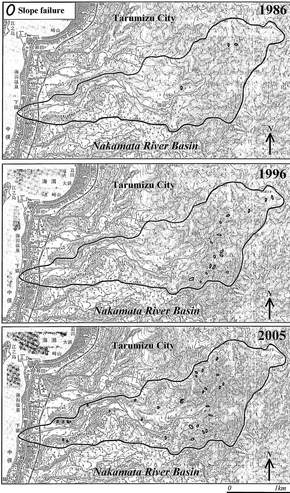
Fig. 2 Distribution charts of slope failure scars based on aerial photographic interpretation.
