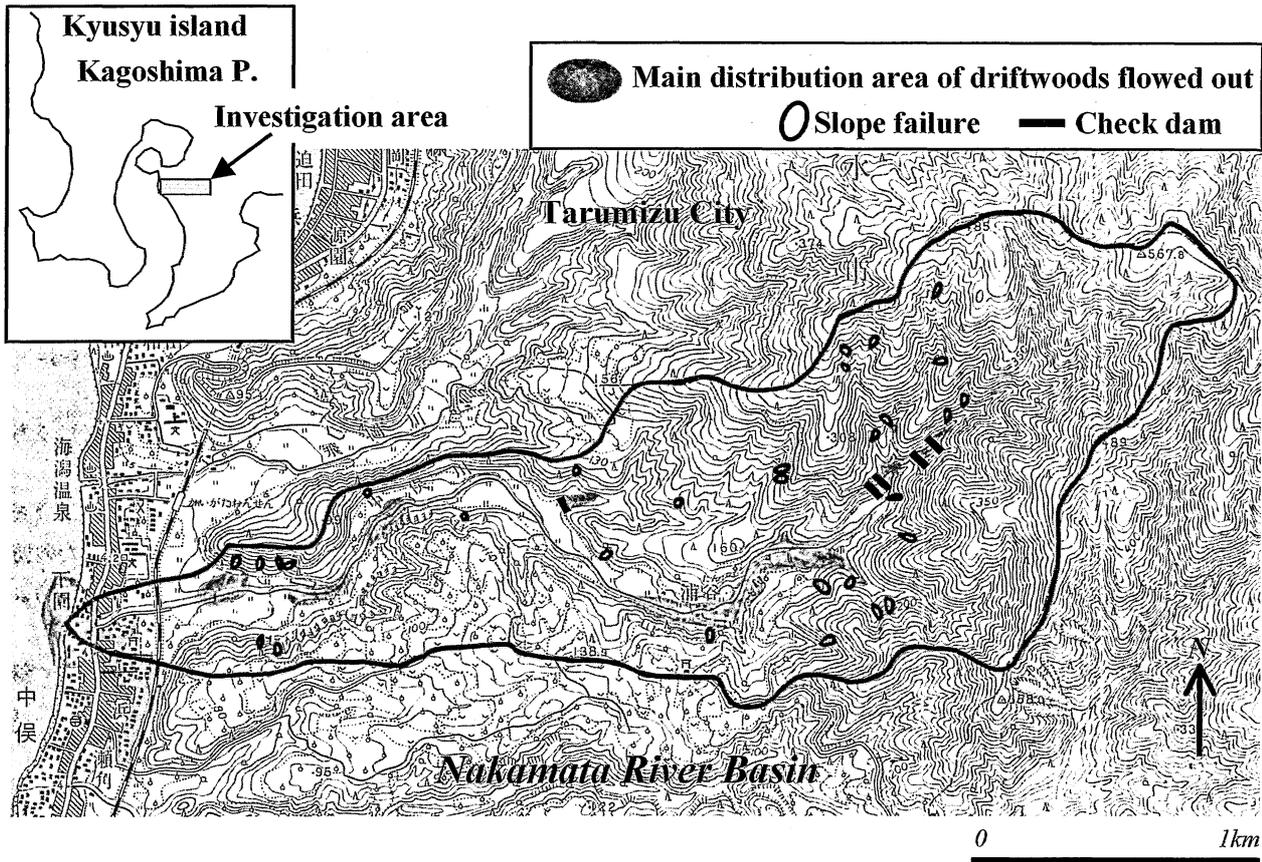
Fig. 6 The main distribution chart of driftwoods flowing out of the Nakamata River Basin based on a field investigation.
