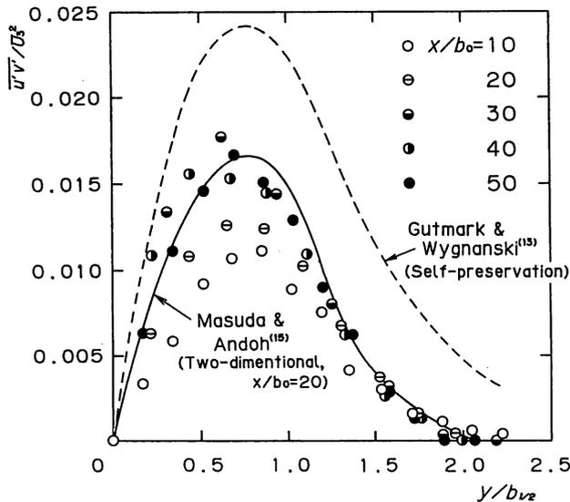
Fig. 4 Reynolds shear stress
