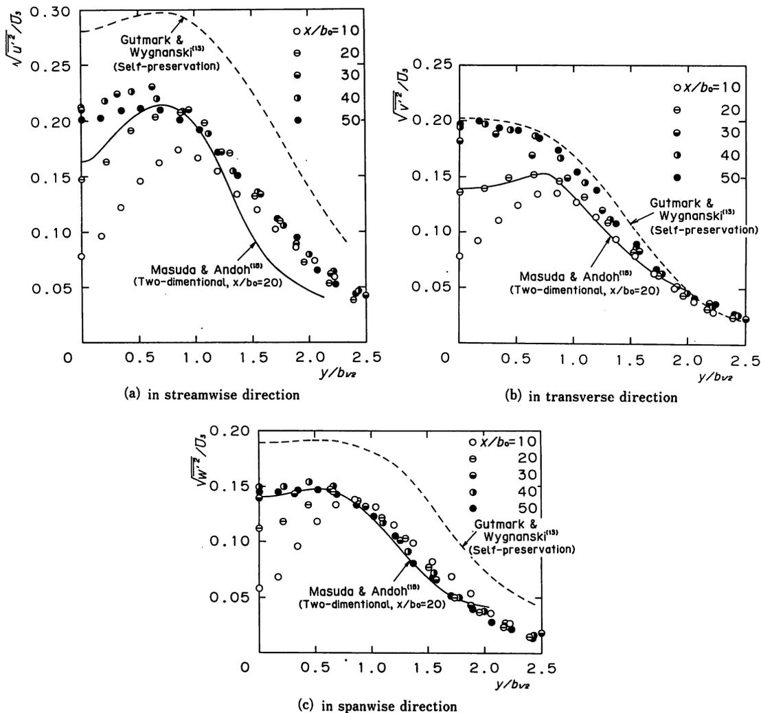
Fig. 3 Streamwise variation of the turbulence intensity
