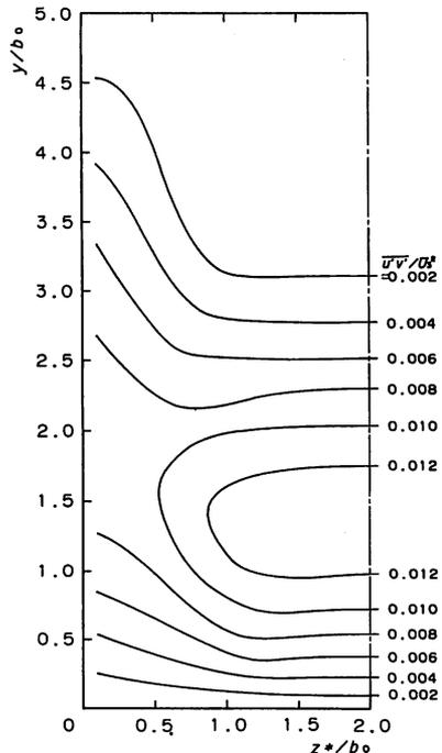
Fig. 10 Contour lines of the Reynolds shear stress ( $x/b_0 = 20$ )
