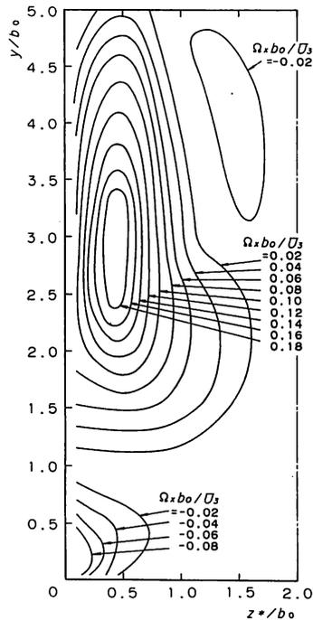
Fig. 11 Contour lines of the vorticity ( $x/b_0 = 20$ )
