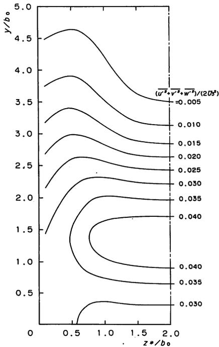
Fig. 9 Contour lines of the turbulence energy ( $x/b_0 = 20$ )
