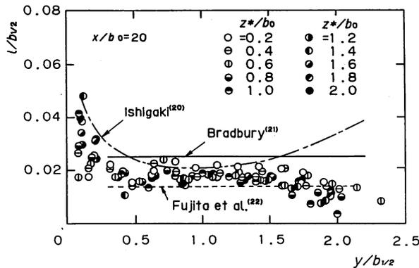
Fig. 7 Spanwise variation of the mixing length
