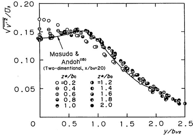
Fig. 6 Similarity of the turbulence intensity in transverse direction
