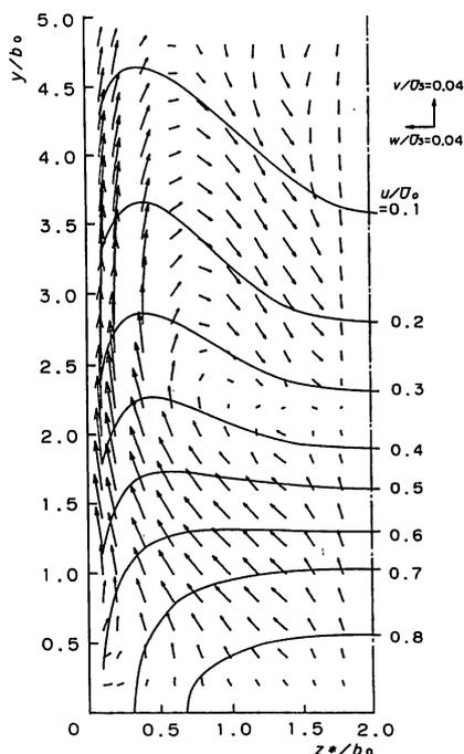
Fig. 8 Secondary flow and the contour lines of the velocity ( $x/b_0 = 20$ )
