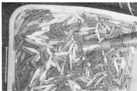
Fig. 2. Model fishes, made of rubber balloons inflated with salt water.
