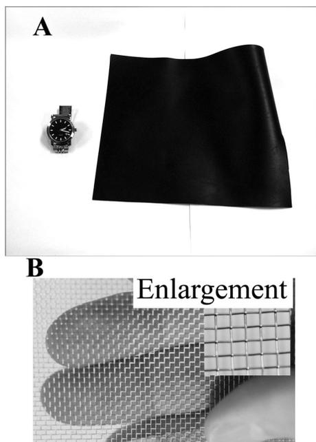
Fig. 8. Photographs of underwater curtain used in the present study. A, rubber curtain; B, net curtain.
