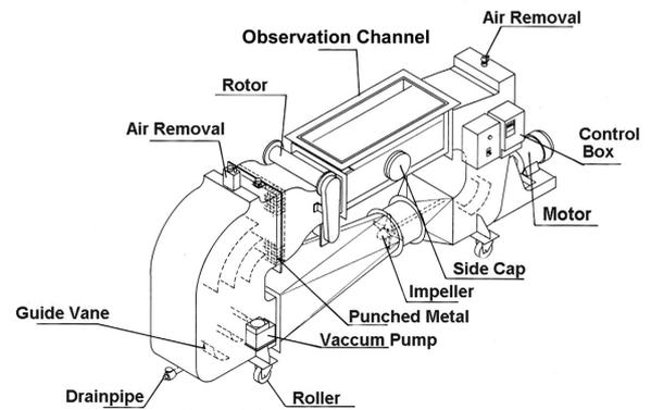
Fig. 5. Schematic of the circulating water channel used in the present study. An observation section is 1.3 m long, 0.3 m wide and 0.2 m deep.
