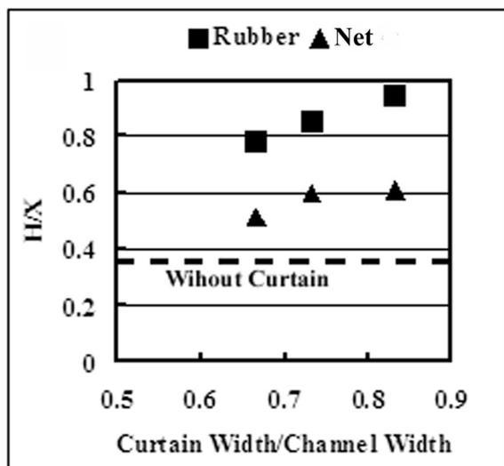
Fig. 15. Diagram of  $H/X$  versus ratio of curtain width to channel width, showing channel wall effect on the experimental results.
