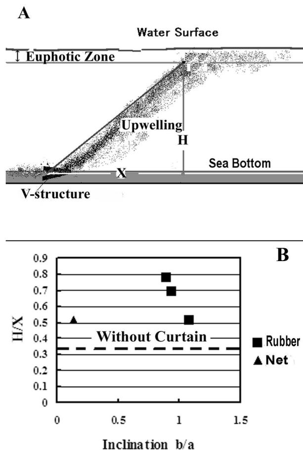
Fig. 11. A: Definition of effectiveness of artificial upwelling device by  $H/X$ . Larger  $H/X$  indicates steeper ascendance of upwelling. B: Diagram of  $H/X$  versus curtain inclination  $b/a$  for rubber and net curtains.
