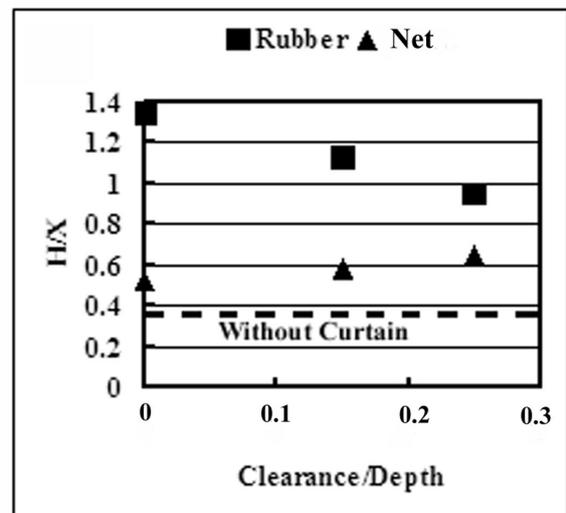
**Fig. 13.** Diagram of  $H/X$  versus curtain-buoy clearance, showing that  $H/X$  decreases with clearance by using a rubber curtain, while  $H/X$  increases very slightly with clearance by using a net curtain.
