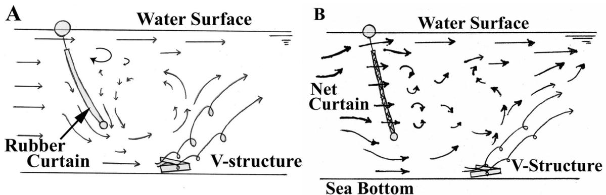
**Fig. 14.** A: Schematic of flow pattern behind rubber curtain with curtain-buoy clearance, showing separation zone reduced as compared with Figure 12-A. B: Schematic of flow pattern behind net curtain with curtain-buoy clearance.
