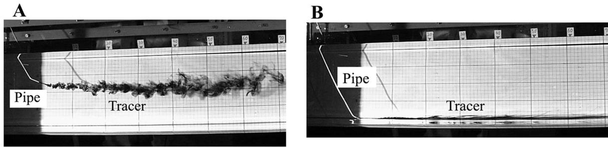
**Fig. 9.** A: Behavior of the tracer in uniform flow, showing that the specific density of the tracer is nearly equal to that of fresh water. B: Tracer's behavior near channel bottom without any obstacles, showing no ascending flow.
