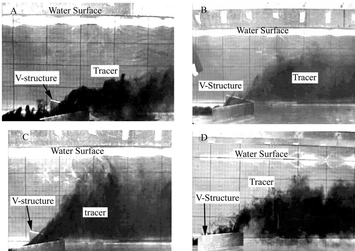
**Fig. 10.** Flow visualization test results for artificial upwelling device. A, V-shaped structure only; B, rubber curtain model with larger curtain inclination and V-shaped structure; C, rubber curtain model with smaller curtain inclination and V-shaped structure; D, net curtain model and V-shaped structure.
