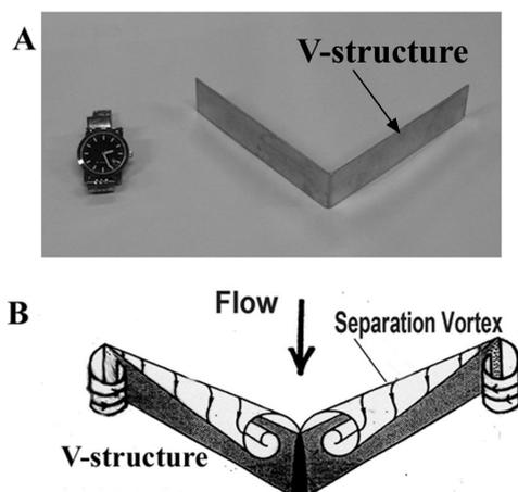
Fig. 1. A: V-shaped upwelling structure model used in the present study. B: Illustration of separation vortices issued from top edge of the V-shaped structure when bottom flow gets over the V-shaped structure installed on the sea bottom.
