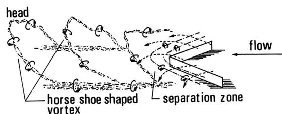
Fig. 2. Illustration of flow pattern behind a V-shaped structure cited from Asaeda (1989).
