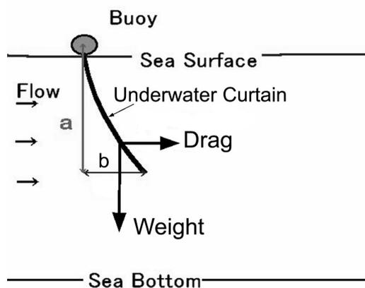
Fig. 7. Definition of curtain inclination, which is dependent on the ratio of hydrodynamic drag of underwater curtain to the curtain weight.
