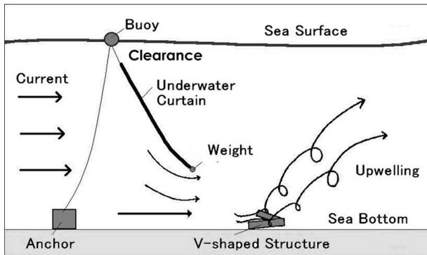
Fig. 4. Schematic of new artificial upwelling device, which is a combined V-shaped structure with vertical flexible underwater curtain hung from floating buoys.
