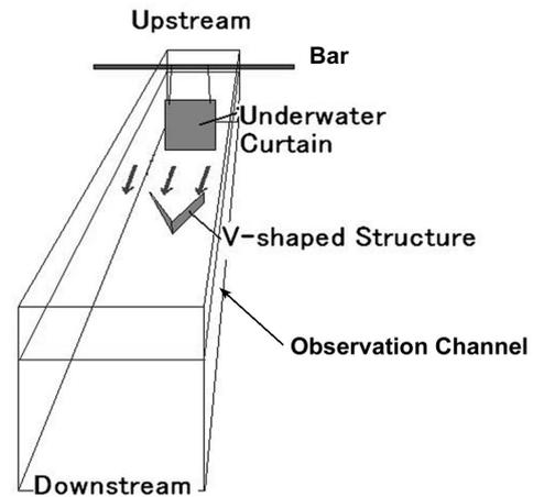
Fig. 6. Schematic of test arrangement in the circulating water channel, showing positions of V-shaped structure model and underwater curtain in the channel, and water flow from upstream to downstream.
