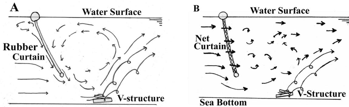
**Fig. 12.** A: Schematic of flow pattern behind rubber curtain showing existence of large separation zone, which results in steeper upwelling. B: Schematic of flow pattern behind net curtain showing velocity reduction due to passage through net mesh.
