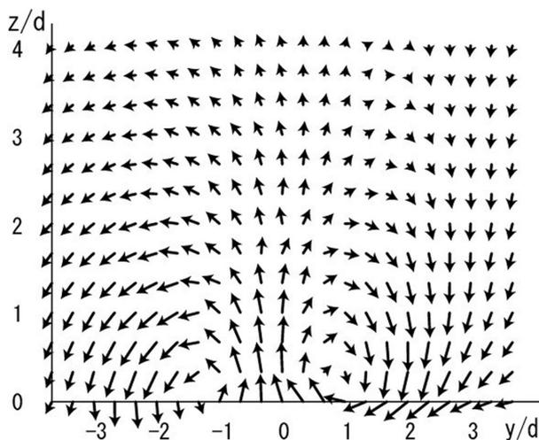
Fig. 3. Velocity vectors measured at a vertical section behind a V-shaped structure cited from Nagamatsu *et al.* (2003), which shows a pair of vortices with counter-ward rotation.
