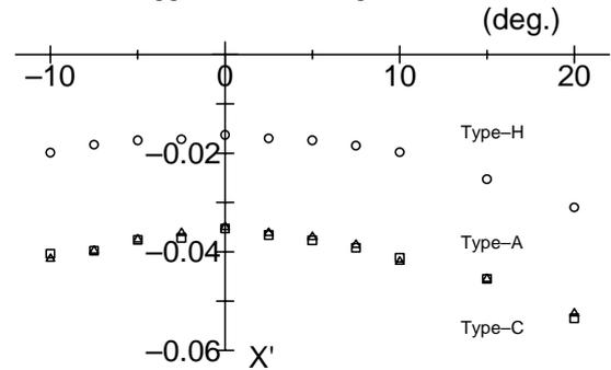
Fig. 4 Non-dimensional resistance acting on the outrigger craft.
