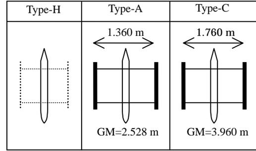
Fig. 3 Schematic illustration of model arrangements.
