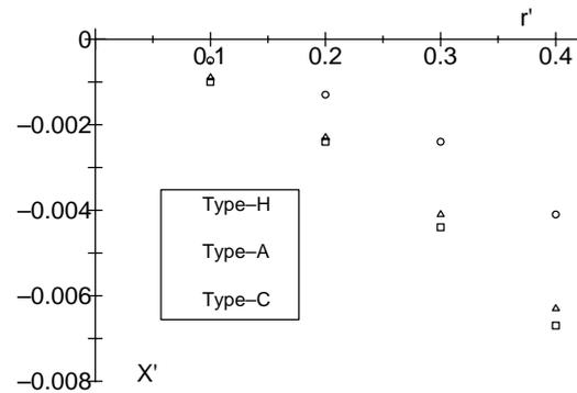
Fig. 5 Increased resistances due to the angular velocity of yawing.
