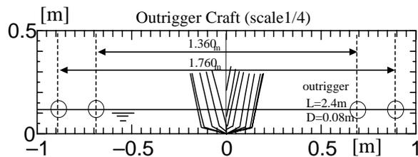
Fig. 2 Body plan of the outrigger craft.
