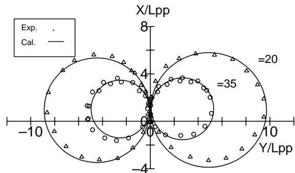
Fig. 10 Turning trajectories on the outrigger craft with a 1.36 m beam in length (Type-A).
