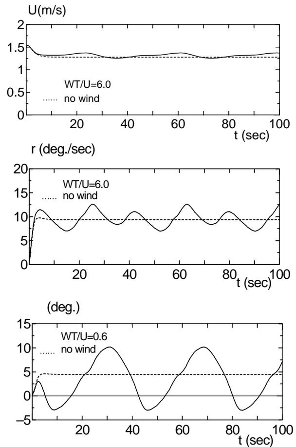
Fig. 15 Time histories of ship's speed  $u$ , yaw rate  $r$  and drift angle  $\beta$  in turning motion under wind force (type-C, rudder angles of 35 degrees).
