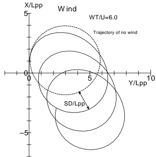
Fig. 14 Example of simulation results of turning trajectories under wind force (type-C, rudder angles of 35 degrees).
