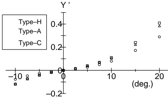
Fig. 6 Lateral forces of the outrigger craft due to oblique motions.
