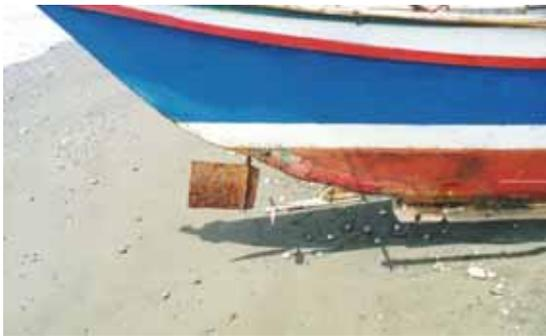
Photo. 1 Rudder and propeller of outrigger craft
