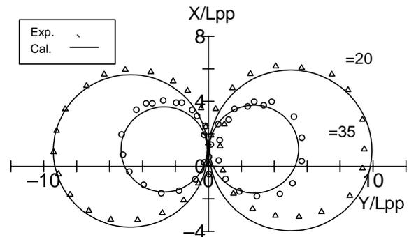
Fig. 11 Turning trajectories on the outrigger craft with a 1.76 m beam in length (Type-C).
