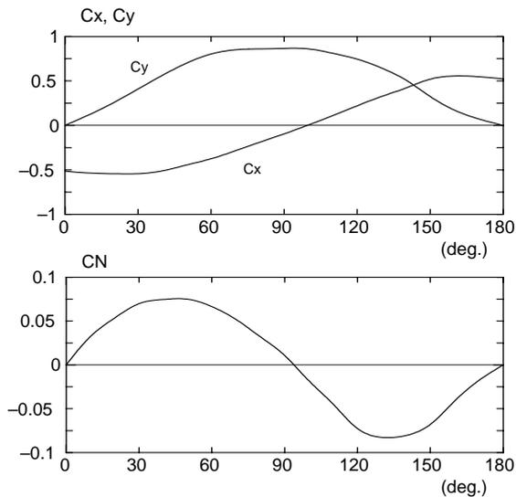
Fig. 12 Coefficients of wind force and moment.
