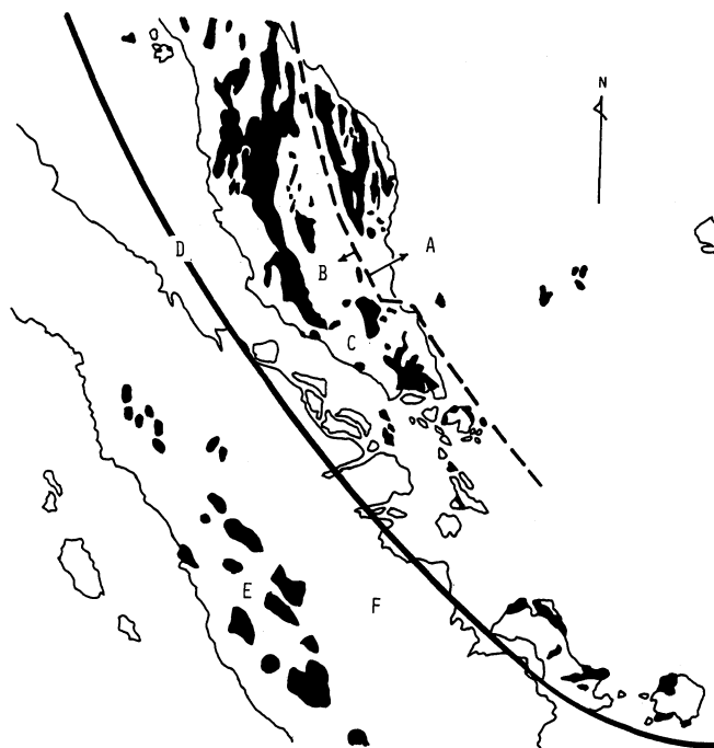
Fig. 2. Distribution of isolated granite plutons associated with tin deposits in Malay Peninsula and Sumatra. Modified in part and simplified from an original figure of HUTCHISON (1973). A, Granite generally of upper Carboniferous; B, granite generally of late Triassic; C, Malay Peninsula; D, Thai-Malayan orogen; E, middle Cretaceous granite; F, Sumatra.
